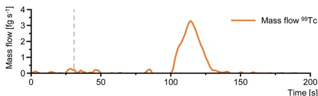
Fig. 7 Mass flow of  $^{99}\text{Tc}$  from analyzing a wastewater sample from a retention basin of the University Hospital of Münster with the combined method consisting of the manual ExC filter disk workflow followed by the automated on-line ExC-IC-ICP-MS method.
