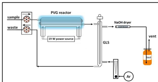
Fig. 2 Schematic of photolysis and gas collection system.
