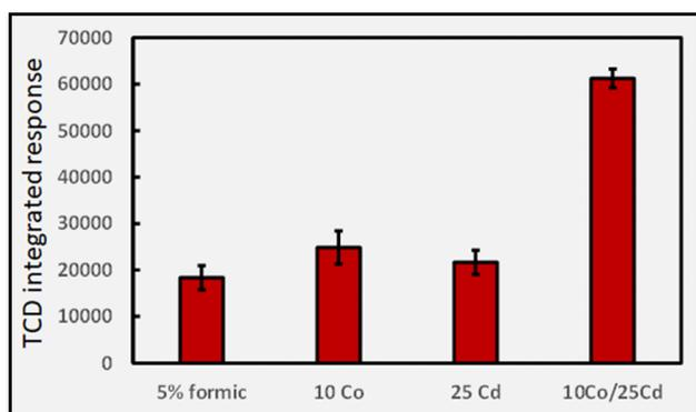
Fig. 11 Synergistic effect of the simultaneous presence of two TMs (concentrations given as  $\mu\text{g mL}^{-1}$ ) on HS  $\text{H}_2$  response (generation) during photolysis of 5% (v/v) formic acid at a solution flow rate of  $2 \text{ mL min}^{-1}$  (IT = 22 s; repeatability SD,  $n = 3$ ). Ordinate displays integrated response characterizing chromatographic peaks.
