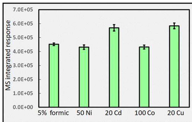
Fig. 12 Impact of added TMs (concentrations given in  $\mu\text{g mL}^{-1}$ ) on HS  $\text{CO}_2$  response (generation) during photolysis of 5% (v/v) formic acid at a solution flow rate of  $2 \text{ mL min}^{-1}$  (IT = 22 s; repeatability SD,  $n = 3$ ). Ordinate units are integrated response over chromatographic peak.
