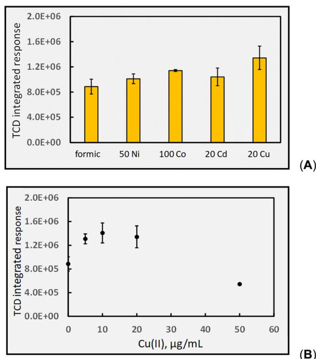
Fig. 9 Impact of added TMs (TM concentrations given as μg mL<sup>-1</sup>) on HS CO response (generation). Photolysis of 5% (v/v) formic acid at a solution flow rate of 2 mL min<sup>-1</sup> (IT = 22 s). Ordinate displays integrated response characterizing chromatographic peaks. (A) Uncorrected HS [CO] increases from 4290 ± 570 ppm to 6550 ± 900 ppm (repeatability SD, *n* = 3) in the presence of 20 μg mL<sup>-1</sup> Cu(II). (B) Effect of increasing Cu(II) on HS CO response (generation).
