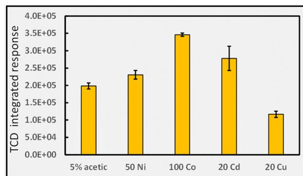
Fig. 13 Impact of added TMs (concentrations given as  $\mu\text{g mL}^{-1}$ ) on HS  $\text{CH}_4$  response (generation) from photolysis of 5% (v/v) acetic acid at  $2 \text{ mL min}^{-1}$  (IT = 32 s; repeatability SD,  $n = 3$ ). Ordinate displays integrated response characterizing chromatographic peaks.
