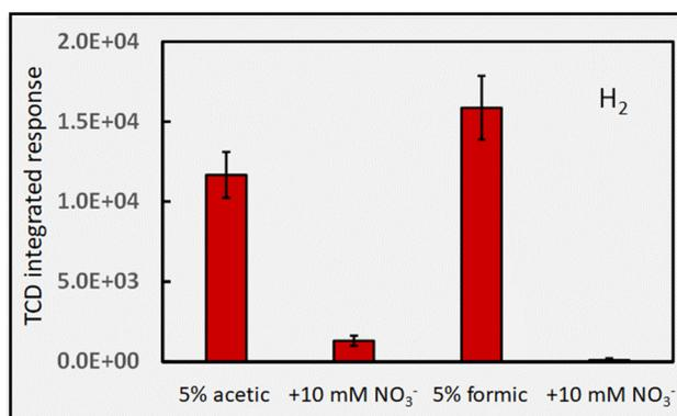
Fig. 8 Impact of the presence of 10 mM  $\text{NO}_3^-$  on HS  $\text{H}_2$  response (generation) during photolysis of 5% (v/v) formic and acetic acids at 2 mL min<sup>-1</sup> (IT = 22 s). Repeatability SD,  $n = 3$ . Ordinate displays integrated response characterizing chromatographic peaks.
