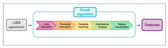
Fig. 2 Processing pipeline of the comb algorithm.
