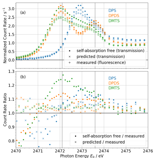
Fig. 6 (a) NEXAFS spectra of dipropyl sulfide (DPS, blue), dipropyl disulfide (DPDS, orange) and dimethyl trisulfide (DMTS, green). The self-absorption free (undamped) spectra, directly calculated from transmission measurements, are depicted with dots, the measured fluorescence spectra are marked with pluses, and the crosses in between are the forward calculated fluorescence spectra predicted using transmission and tabulated data. (b) The residues for the measured transmission and the predicted fluorescence spectra relative to the measured fluorescence spectra visualize that the forward calculation makes up for the damping of the NEXAFS signal and especially recovers the peak height ratios in the damped fluorescence spectra. The full data over the whole energy axis are shown in the ESI.†
