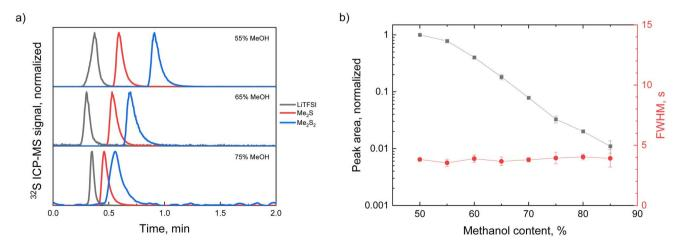
Fig. 1 (a) LC-ICP-MS chromatograms of LiTFSI, Me<sub>2</sub>S and Me<sub>2</sub>S<sub>2</sub> standards (separate injections) acquired using different methanol contents in the eluent (55%, 65% and 75%); (b) normalized response factor measured as peak area and the peak width (full width at half-maximum, FWHM) of the Me<sub>2</sub>S signal at various methanol contents in the eluent. The Ar sample gas flow value was 0.7 L min<sup>-1</sup> and the eluent flow was 0.5 mL min<sup>-1</sup>.
