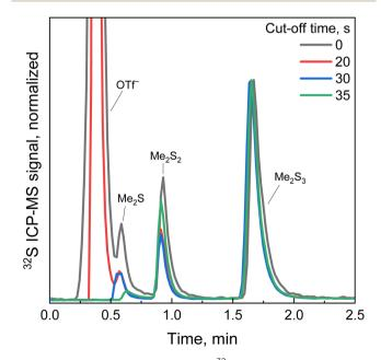
Fig. 3 HPLC-ICP-MS chromatograms ( $^{32}$ S) normalized to the signal of Me<sub>2</sub>S<sub>3</sub> of a derivatized mixture with a nominal composition Li<sub>2</sub>S<sub>3.8</sub> with a cut of the signal of LiOTf at 20, 30, and 35 s after injection as well as the chromatogram with no diverted flow (black solid line).
