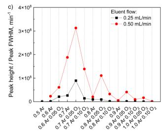
Fig. 2 Peak width (a), signal-to-noise ratio (b) and sharpness (c) of the dimethyl sulfide signal collected in the HPLC-ICP-MS experiment for various eluent flows and sample gas flows with 55% methanol in the eluent. No chromatography peak is observed for  $0.5~\mathrm{mL}~\mathrm{min}^{-1}$  eluent flow with  $0.5 L min^{-1}$  sample gas flow.
