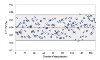
Fig. 7 Long-term reproducibility of the  $\delta^{114/110}$ Cd measurement value for NIST SRM 3108 at 10 ng mL $^{-1}$  over five months. The grey area represents  $\pm 2$ SD (n=170).
