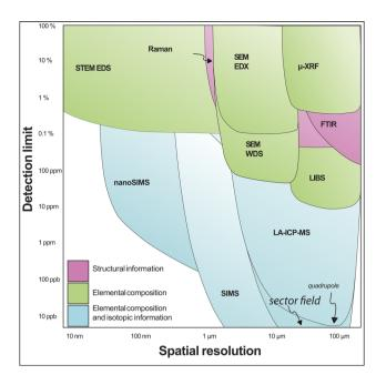
Fig. 1 Detection limit vs. spatial resolution (x-axis) for the suite of microbeam methods commonly utilised by geoscientists, adapted from Chew et al.<sup>26</sup> and Li and Li.<sup>27</sup>
