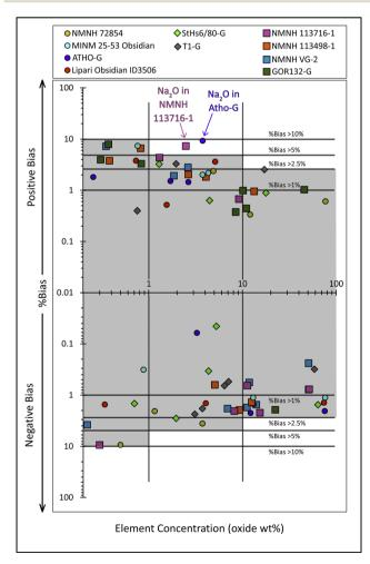
Fig. 6 Spot analysis on a suite of natural glasses (ESI Table 1†) displaying the accuracy using a scanning FoV of 5  $\mu$ m and for 1M counts. Shaded area outlines analysis within error.
