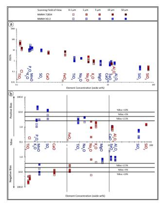
Spot analyses on basaltic glass NMNH VG-2 and rhyolitic glass NMNH 72854 collected for a range of field of views to determine the optimal scanning FoV required for best precision (a) and accuracy (b). The full dataset is found in ESI Table 1.†
