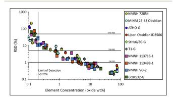
Fig. 5 Spot analysis on a suite of natural glasses (ESI Table 1†) displaying the precision using a scanning FoV of 5 µm and for 1M counts.
