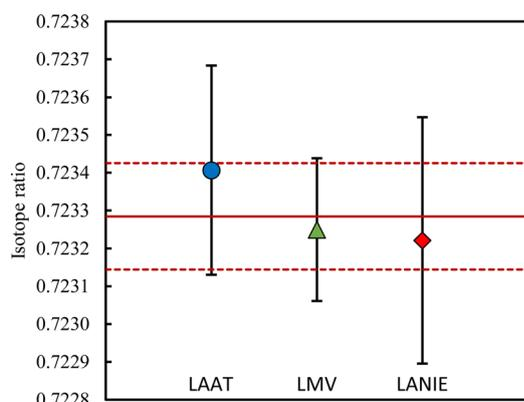
Fig. 3  $^{146}\text{Nd}/^{144}\text{Nd}$  isotope ratio and its expanded uncertainty measured by the LAAT (blue circle), LANIE (red diamond) and LMV (green triangle) laboratories. The red line corresponds to the final average value with its expanded uncertainty (red dotted line).
