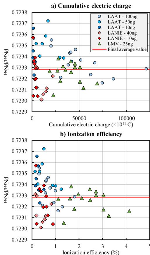
Fig. 2  $^{146}\text{Nd}/^{144}\text{Nd}$  isotope ratio as function of the cumulative electric charge on all Nd isotopes (a) and as function of the ionization efficiency (b) by the LAAT (blue circle), LANIE (red diamond) and LMV (green triangle) laboratories and for different quantities.
