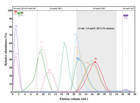
Fig. 1 Elution curve for Ni purification in the first column with 2 mL AG50W-X8 (200–400 mesh) cation resin. The igneous reference material BHVO-2 was utilized with 2.6  $\mu$ g of Ni loaded to generate the elution curve. The shaded area denotes the collection Ni elution part.
