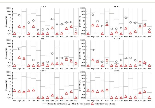
Fig. 2 The residual matrix element contents relative to Ni content (i.e., [element]/[Ni] ratios before the purification (horizontal lines), after the first column (hollow circle points) and the whole scheme (hollow triangular points)). Y = 0.001 indicates [element]/[Ni] ratios ≤0.001. The horizontal title element \* refers to the corresponding matrix element
