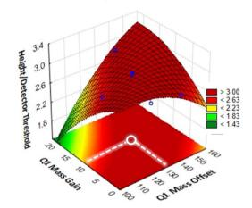
Fig. 1 Colorimetric maps obtained from the Doehlert experimental design for (A) plasma and (B) bandpass optimisations. Selected conditions are marked as a white circle
