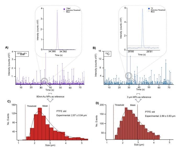
Fig. 3 PTFE standard (3  $\mu$ m) characterisation via F and C SP analysis. (A) and (B) Show SP events detected for  $^{157}$ BaF<sup>+</sup> and  $^{12}$ C<sup>+</sup>,respectively. A magnification for one selected SP event is provided on the top. (C) and (D) Show the calibrated size distributions, respectively.
