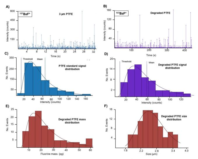
Fig. 4 (A) Raw SP ICP-MS monitoring BaF<sup>+</sup> found in the 3 µm PTFE standard suspension. (B) BaF<sup>+</sup> ion events detected in a degraded PTFE sample, (C) 3 µm PTFE standard signal distribution, (D) signal histograms from the degraded PTFE sample, (E) histogram representing the fluorine mass (pg) per particle and (F) size histogram (µm) of the detected F-based particles in the degraded PTFE sample.
