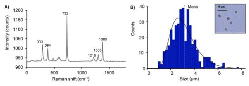
Fig. 2 (A) Raman spectrum obtained from the 3 μm PTFE standard, (B) size histogram and optical image of the detected particles.
