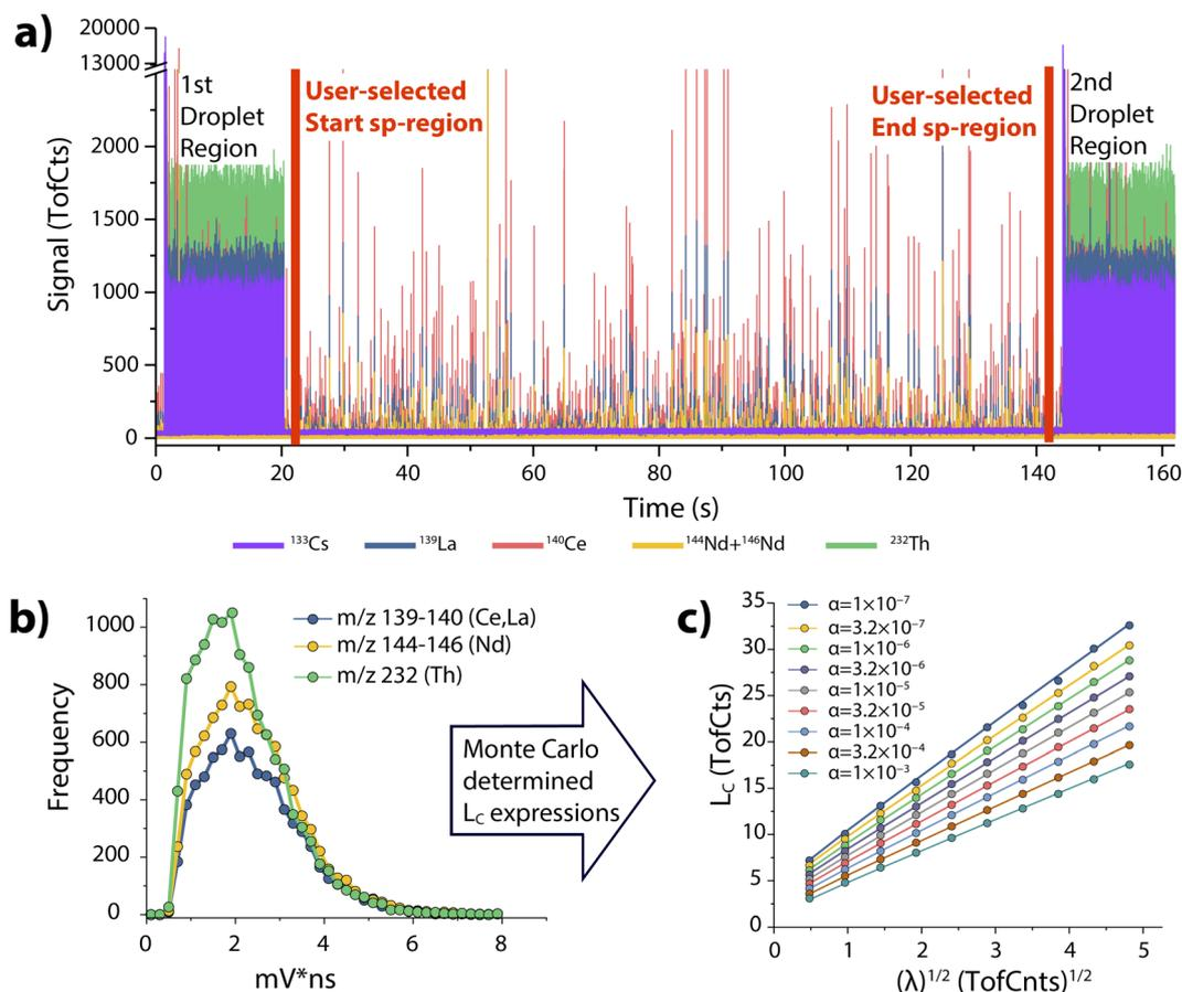
Fig. 2 (a) In the first step of TOF-SPI, the user identifies the start and end points of the sp-region on the ICP-TOFMS time trace, which separate the droplet regions from the region with only particle-derived signals. (b) The user also loads and/or selects the TOF signal-ion-signal (SIS) histogram for the day's measurements and (c) TOF-SPI constructs mass-dependent critical value ( $L_C$ ) expressions based on Poisson-distributed ion signals compounded with the SIS noise.
