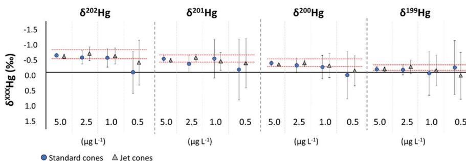
Fig. 2 Average  $\delta^{XXX}\text{Hg}$  (‰) values for the IH standard ( $n = 5$ ) obtained at different concentration levels with standard and jet cones under wet plasma conditions and using  $10^{11} \Omega$  amplifiers. Red dashed lines represent the average  $\pm 2\text{SD}$  for previously obtained IH values.<sup>6</sup> Error bars correspond to  $2\text{SD}$  and are obtained from  $n = 5$  CVG-MC-ICP-MS measurements.
