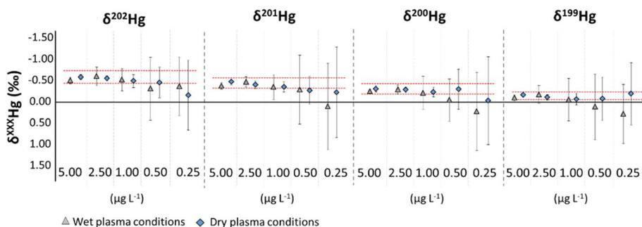
Fig. 3 Average  $\delta^{\text{XXX}}\text{Hg}$  (‰) values for the IH solution ( $n = 5$ ) obtained at different concentration levels under wet and dry plasma conditions using  $10^{11}\ \Omega$  amplifiers and jet cones. Red dashed lines represent the average  $\pm 2\text{SD}$  of the previously obtained IH values.<sup>6</sup> Error bars correspond to 2SD and are obtained from  $n = 5$  CVG-MC-ICP-MS measurements.
