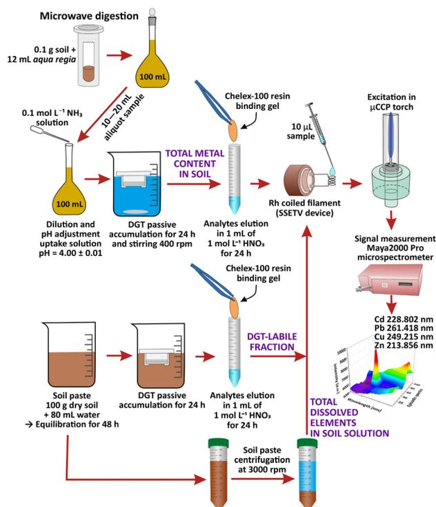
Fig. 1 Schematic diagram of soil sample preparation for the determination of total content and labile fraction of Cd, Pb, Cu and Zn in soil by SSETV- $\mu$ CCP-OES after DGT passive accumulation on Chelex-100 resin.
