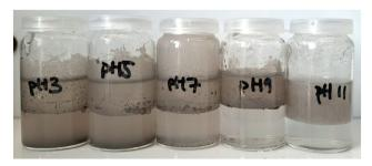
Fig. 5 NiO particle suspensions in two immiscible liquid systems (top: cyclohexane, bottom: DI water at different pH values). From left to right, pH 3, 5, 7, 9, and 11.
