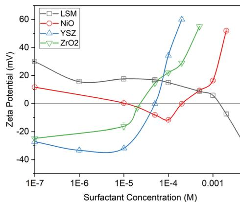
**Fig. 2** Zeta potential of representative materials in the presence of oppositely charged surfactants: SDS (for LSM and NiO) and CTAB (for YSZ and ZrO<sub>2</sub>) at pH 10. The lines are guides for the eye and error bars indicate 95% of confidence interval.
