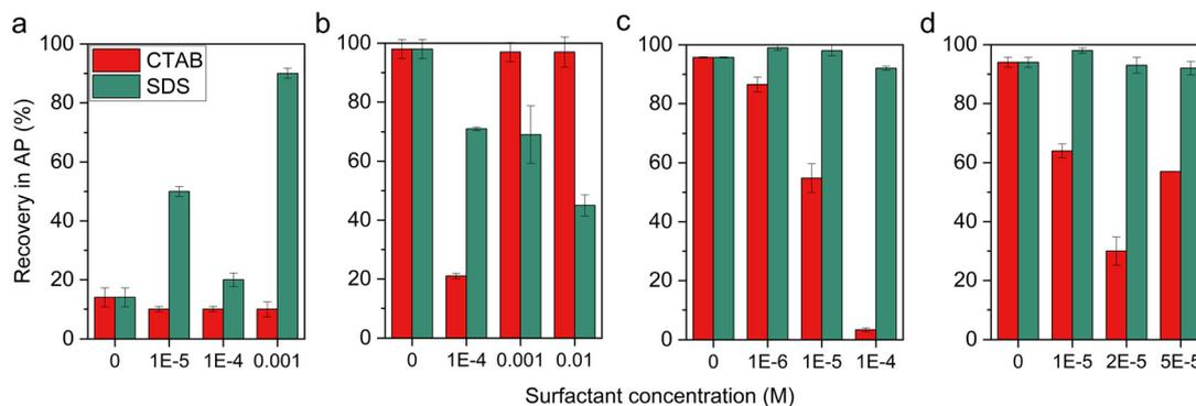
**Fig. 4** Phase separation of the single particle system: (a) NiO; (b) LSM; (c) YSZ; (d) ZrO<sub>2</sub>. The recovered particles in the aqueous phase (AP) subsequent to the surfactant concentration at pH 10 in % (w/w), error bars indicate 95% of confidence interval.
