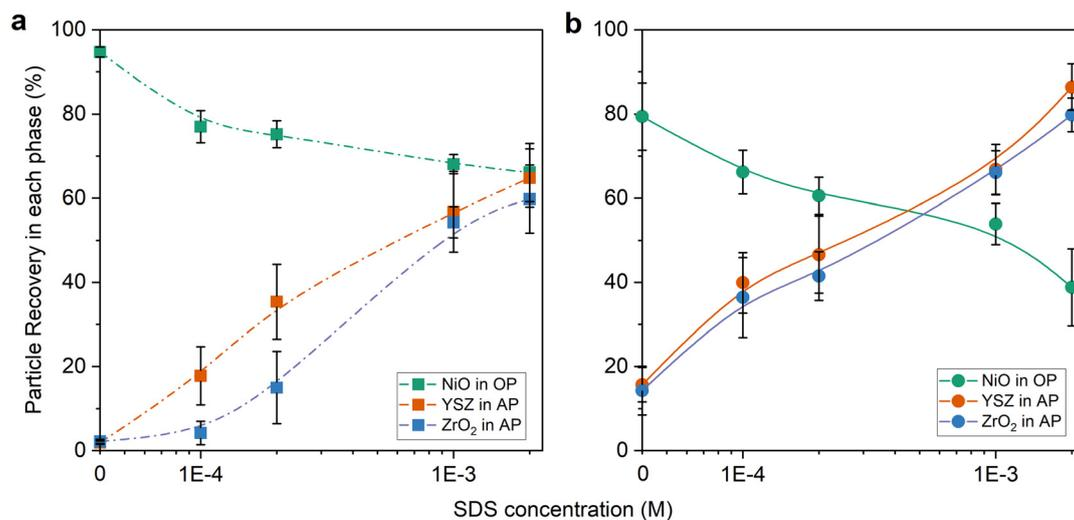
Fig. 7 Mass percentage of the recovered particles in the target phases (NiO in the organic phase (OP) and YSZ and ZrO<sub>2</sub> in the aqueous phase (AP)) by means of LLPS. (a) Without sonication treatment; (b) including a sonication process during experiments. The lines are guides for the eye and the error bars indicate 95% of confidence interval.
