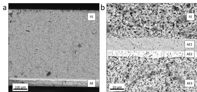
**Fig. 1** Cross sectional back scattered electron scanning electron microscopy (BSE-SEM) images of the HTEL MEA. (a) Magnification of 400; (b) magnification of 4000. FE: fuel side electrode including its substrate layer, AE1: solid electrolyte, AE2: barrier, AE3: air side electrode.
