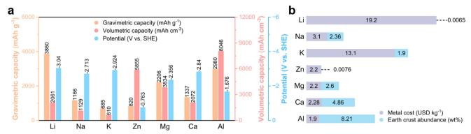
Fig. 1 Advantages of Al as a battery anode. (a) Comparison of theoretical specific capacities and standard electrochemical reduction potentials of different metal anodes. (b) Abundance of different metal elements in the Earth's crust and the cost of metal anodes. Reprinted with permission. 16 Copyright 2021, WILEY-VCH VERLAG GMBH.
