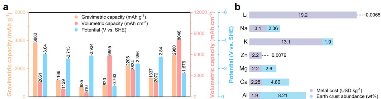
**Fig. 1** Advantages of Al as a battery anode. (a) Comparison of theoretical specific capacities and standard electrochemical reduction potentials of different metal anodes. (b) Abundance of different metal elements in the Earth's crust and the cost of metal anodes. Reprinted with permission.<sup>16</sup> Copyright 2021, WILEY-VCH VERLAG GMBH.
