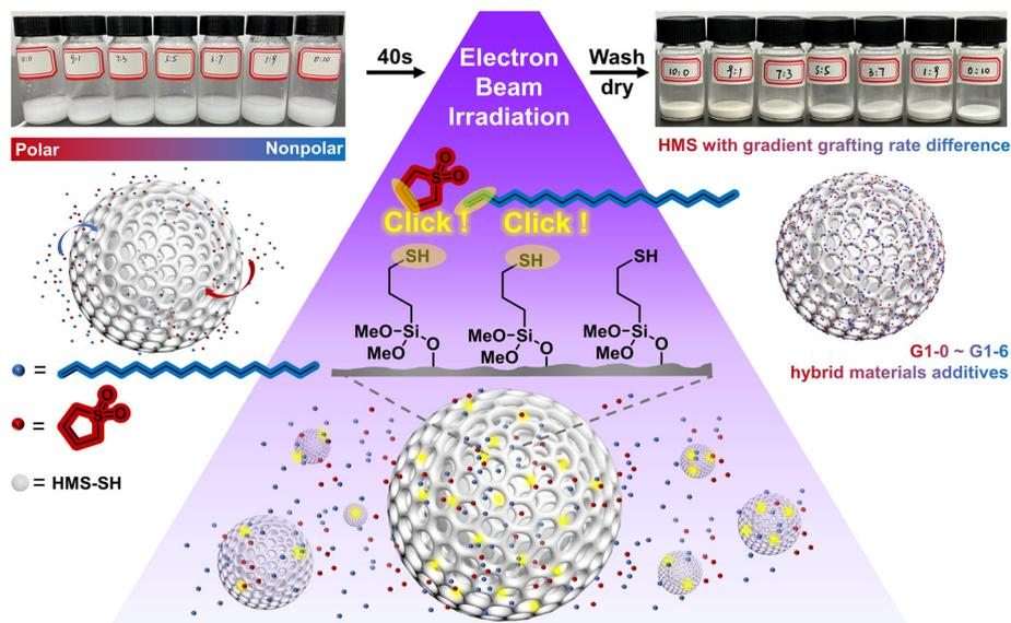
Fig. 13 The general procedure for the preparation of the EBI-grafted hybrid materials of the G1 series.
