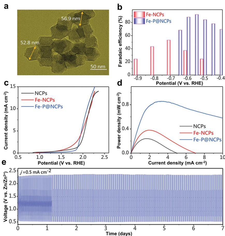
**Fig. 5** (a) TEM image of the synthesized Fe-P@NCPs. (b)  $FE_{CO}$  values at different applied potentials for Fe-NCPs and Fe-P@NCPs. (c) OER evaluation by the LSV curves in a  $0.1$  M  $KHCO_3$  solution. (d) Power density curves of the aqueous Zn-CO<sub>2</sub> cell based on different samples. (e) Galvanostatic discharge-charge cycling curves at  $0.5$  mA cm<sup>-2</sup> for Fe-P@NCPs. Reproduced from ref. 88 with permission from Wiley-VCH, copyright 2022.
