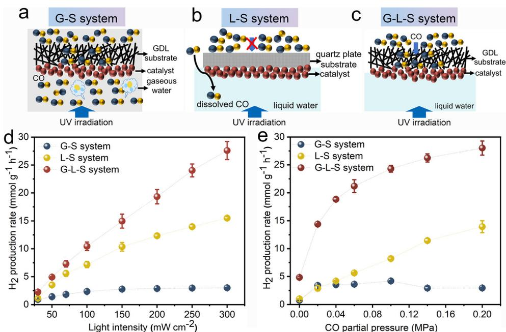
**Fig. 4** Schematic illustration of (a) G-S, (b) L-S, and (c) G-L-S systems; (d) light intensity-dependent photocatalytic H<sub>2</sub> production rate over Rh/TiO<sub>2</sub> at a CO partial pressure of 0.2 MPa; (e) CO partial pressure-dependent photocatalytic H<sub>2</sub> production rate at a light intensity of 300 mW cm<sup>-2</sup>. Error bars represent the standard deviation from at least three independent measurements.
