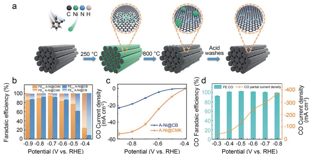
**Fig. 4** (a) Schematic illustration of the synthesis of A-Ni@CMK; (b)  $FE_{CO}$  and  $FE_{H_2}$  of A-Ni@CMK and A-Ni@CB in the H-type cell; (c)  $j_{CO}$  of A-Ni@CMK and A-Ni@CB in the H-type cell; and (d) electrocatalytic activity of A-Ni@CMK in the flow cell.<sup>40</sup> Reprinted with permission from Wiley-VCH, copyright 2021.
