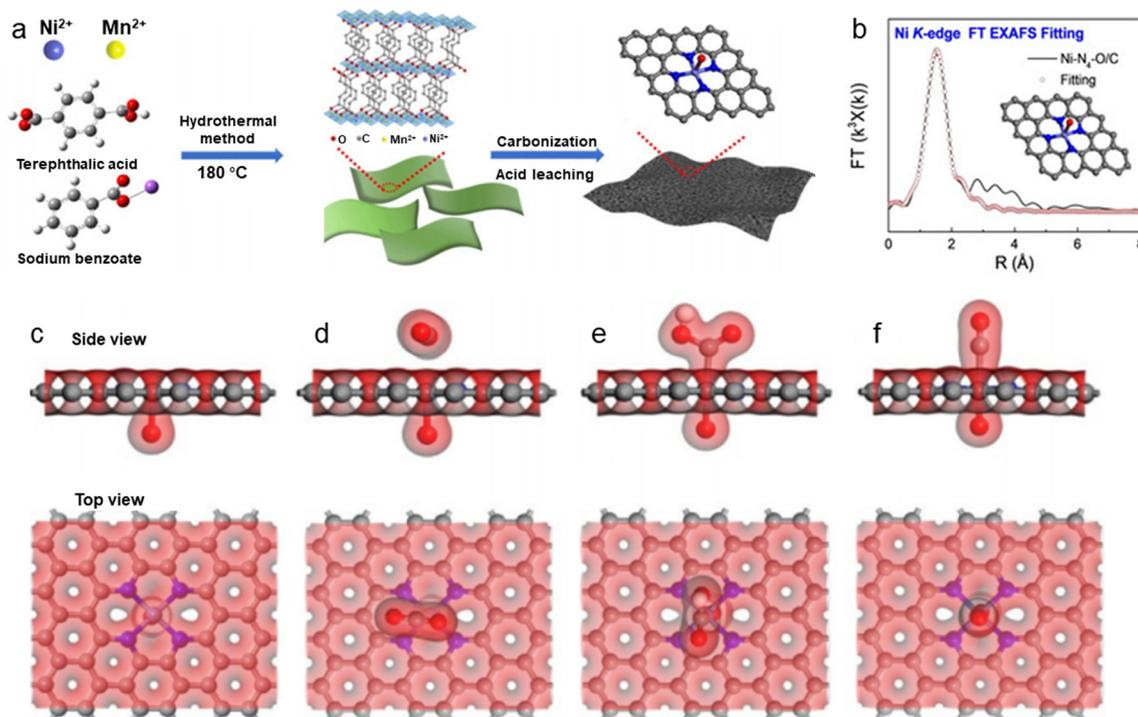
**Fig. 10** (a) Illustration of the synthesis process; (b) EXAFS fitting curves in  $R$  space. Inset: Corresponding schematic model of Ni-N<sub>4</sub>-O/C; (c)–(f) side view and top view of structural evolution of electrochemical CO<sub>2</sub>RR for Ni-N<sub>4</sub>-O/C (Ni cyan, N blue, O red, H white, C grey).<sup>48</sup> Reprinted with permission from Wiley-VCH, copyright 2020.
