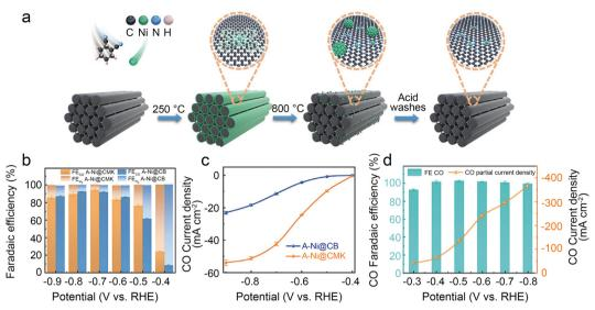
Fig. 4 (a) Schematic illustration of the synthesis of A-Ni@CMK; (b)  $FE_{CO}$  and  $FE_{H_2}$  of A-Ni@CMK and A-Ni@CB in the H-type cell; (c)  $j_{CO}$  of A-Ni@CMK and A-Ni@CB in the H-type cell; and (d) electrocatalytic activity of A-Ni@CMK in the flow cell.<sup>40</sup> Reprinted with permission from Wiley-VCH, copyright 2021.
