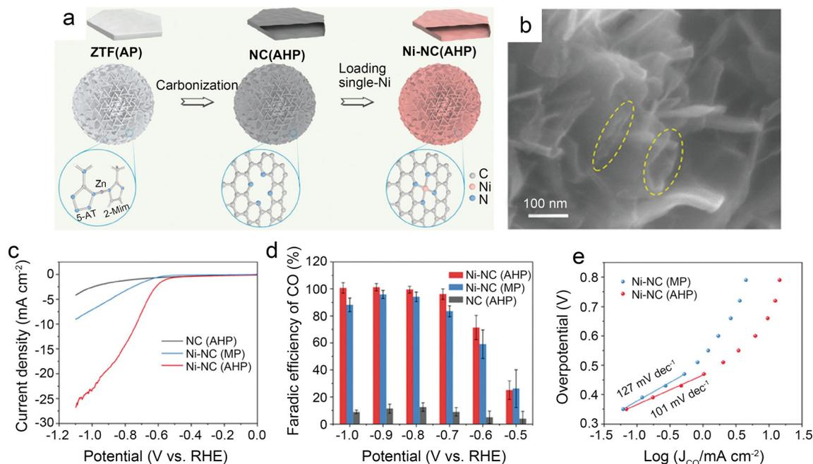
**Fig. 5** (a) Schematic illustration of the preparation route for Ni-NC(AHP); (b) FESEM images of Ni-NC(AHP); the dash circles indicate the openings and parallel walls of hollow plates; (c–e)  $CO_2$  electroreduction performance of samples; (c) LSV curves in  $CO_2$ -saturated  $0.5 \text{ M KHCO}_3$  solution; (d) comparison of  $CO_2$  faradaic efficiency at various potentials; and (e) Tafel plots towards CO product.<sup>41</sup> Reprinted with permission from Wiley-VCH, copyright 2021.
