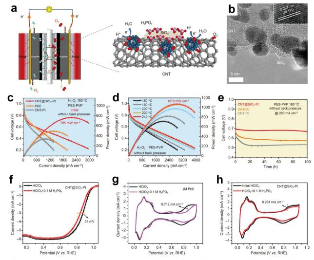
Fig. 7 (a) Single cell and CNT@SiO2-Pt in the catalytic layer of HT-PEMFCs; (b) HR-TEM image of CNT@SiO2-Pt (inset: HRTEM image of CNT@SiO<sub>2</sub>-Pt); (c and d) polarization and power density curves; (e) potential response of a 100 h HT-PEMFCs life test; (f) ORR polarization curves of CNT@SiO<sub>2</sub>-Pt; cyclic voltammograms of (g) JM-Pt/C and (h) CNT@SiO<sub>2</sub>-Pt in N<sub>2</sub>-saturated electrolyte. Reprinted with permission from ref. 47. Copyright 2021, Springer Nature.
