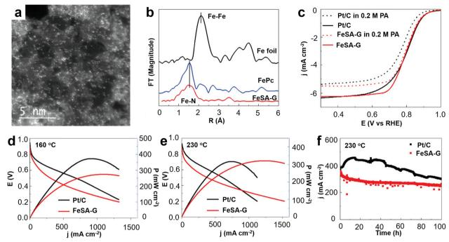
Fig. 14 (a) AC-STEM images for FeSA-G; (b) Fourier transform of the EXAFS spectra of FeSA-G, FePc, and Fe foil; (c) linear scan voltammetry of FeSA-G and Pt/C; J-V and power density curves of high temperature PEMFCs at (d) 160 °C and (e) 230 °C; (f) stability of the cells at 0.5 V. Reprinted with permission from ref. 70. Copyright 2019, John Wiley & Sons.
