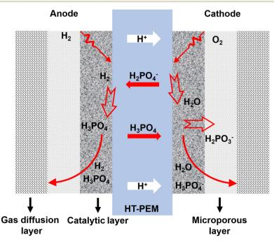
Fig. 1 Distribution and migration of phosphoric acid in membrane electrode.
