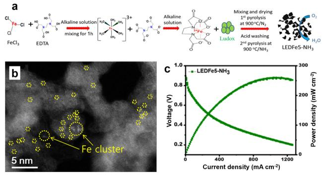
Fig. 12 (a) Schematic illustration of synthesis process for EDTA-Fe complex-based catalyst; (b) HAADF-STEM image of LEDFe<sub>5</sub>-NH<sub>3</sub>; (c) single-cell performance of HT-PEMFC at 1.5 bar O<sub>2</sub> pressure and 150 °C cell temperature. Reprinted with permission from ref. 62. Copyright 2014, American Chemical Society
