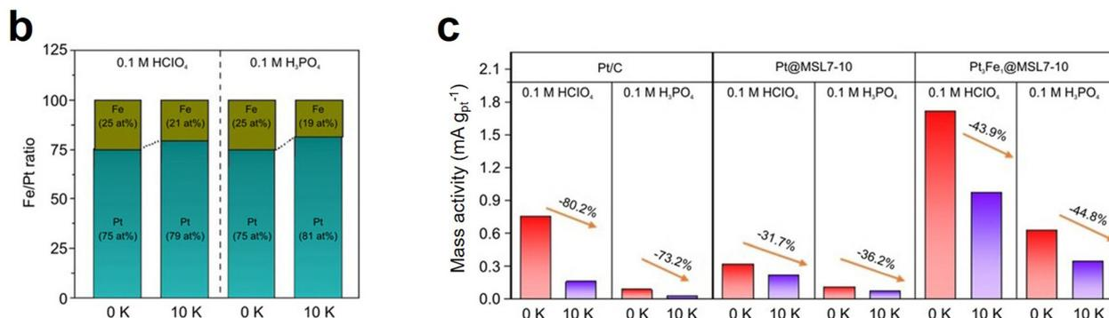
**Fig. 8** (a) Schematic diagram showing the strategy to control the carbon shell structure of Pt-based nanoparticles for realizing the molecular sieve layer effect; (b) Pt/Fe ratios of Pt<sub>3</sub>Fe<sub>1</sub>@MSL7-10 after ADTs; (c) changes in the mass activity of catalysts before and after ADTs. Reprinted with permission from ref. 48. Copyright 2023, John Wiley & Sons.
