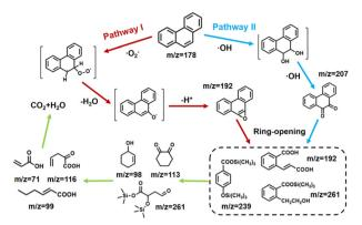
**Fig. 6** Possible degradation pathways of PHE by the piezocatalysis of HAP@FAP-1.5.
