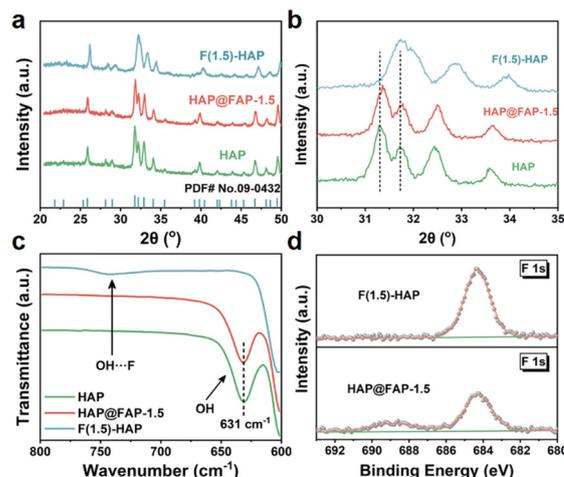
Fig. 3 (a) The XRD patterns of HAP, HAP@FAP-1.5, and F(1.5)-HAP; (b) enlarged view between  $30\text{--}35^\circ$ ; (c) FTIR scans of HAP, HAP@FAP-1.5, and F(1.5)-HAP; and (d) F 1s high-resolution XPS spectra of HAP@FAP-1.5 and F(1.5)-HAP.
