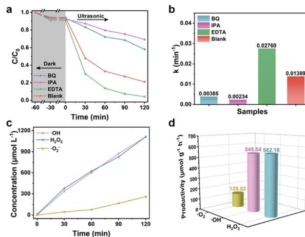
Fig. 8 The effect of scavengers on piezocatalysis with HAP@FAP-1.5 for (a) the degradation of PHE; (b) corresponding degradation kinetic rate constants ( $\text{min}^{-1}$ ); (c) concentration change curves of  $\cdot\text{O}_2^-$ ,  $\cdot\text{OH}$ , and  $\text{H}_2\text{O}_2$ ; (d) corresponding productivities in 120 min under ultrasound.
