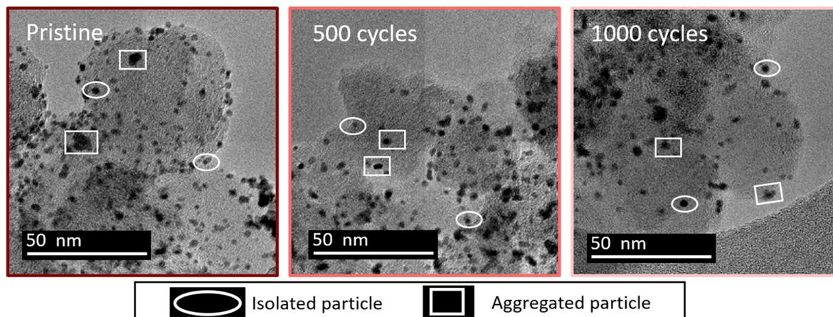
**Fig. 1** Representative TEM images of platinum nanoparticles from a Pt/C 20% TTK at  $20 \mu\text{g cm}^{-2}$  loading at different stages of cycling between 1.2 and 0.4 V vs. RHE in 1 M  $\text{H}_2\text{SO}_4$  + 0.01 M NaCl. The ellipses highlight some examples of isolated particles and the rectangles show some examples of aggregated particles.
