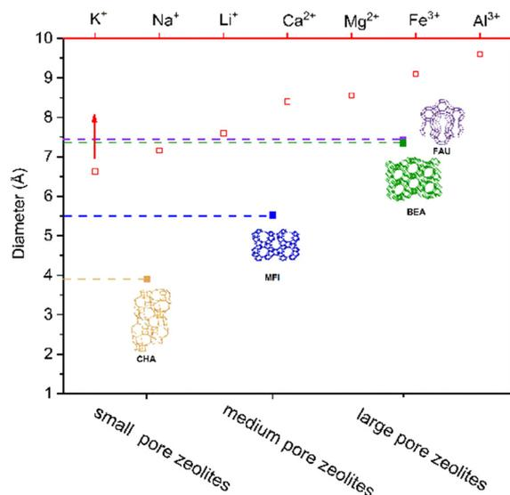
Fig. 4 The relationship between the diameter of metal hydrated ions and the pore size of zeolites.
