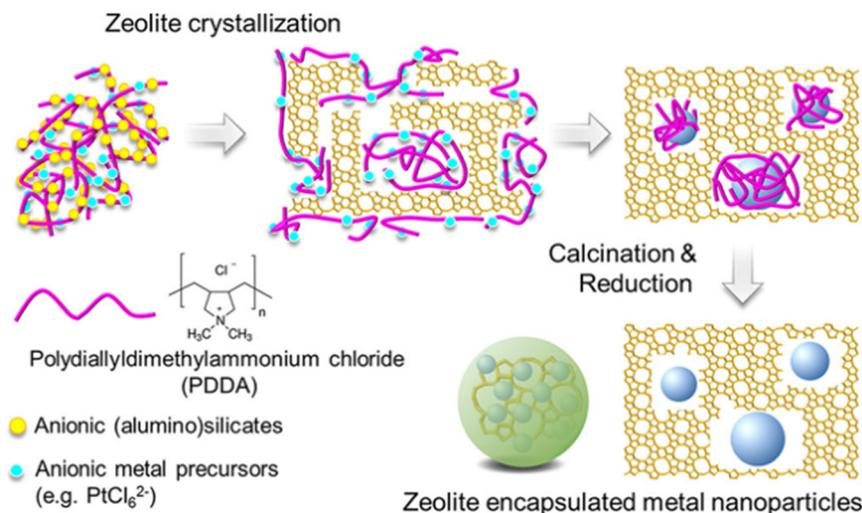
Fig. 7 Synthesis of the polymer-assisted Pd@HZSM-5 catalyst.<sup>26</sup> Reprinted with permission from American Chemical Society, copyright 2018.
