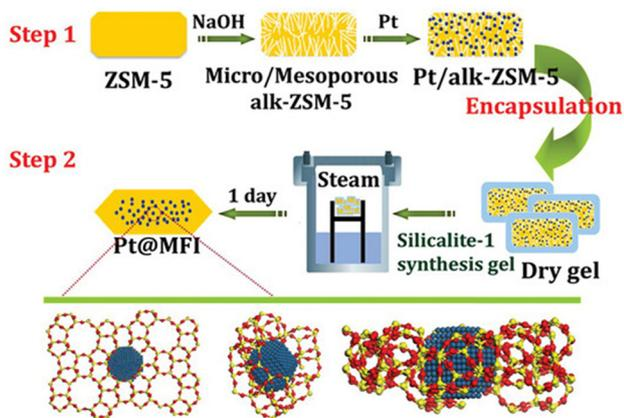
**Fig. 2** Scheme of synthesis of MFI zeolite-encapsulated Pt nanoparticles.<sup>65</sup> Reprinted with permission from American Chemical Society, copyright 2015.
