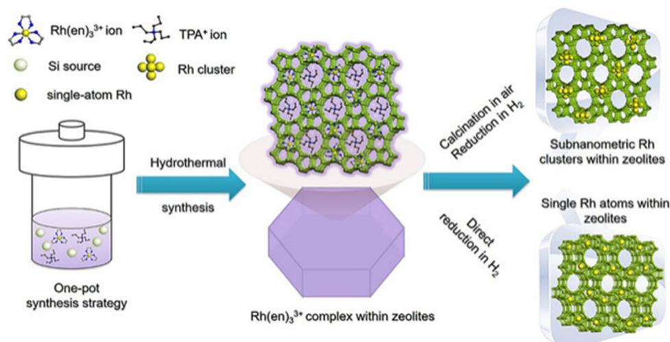
Fig. 5 Schematic of the synthesis of the Rh@S-1 catalyst.<sup>77</sup> Reprinted with permission from Wiley-VCH, copyright 2019.
