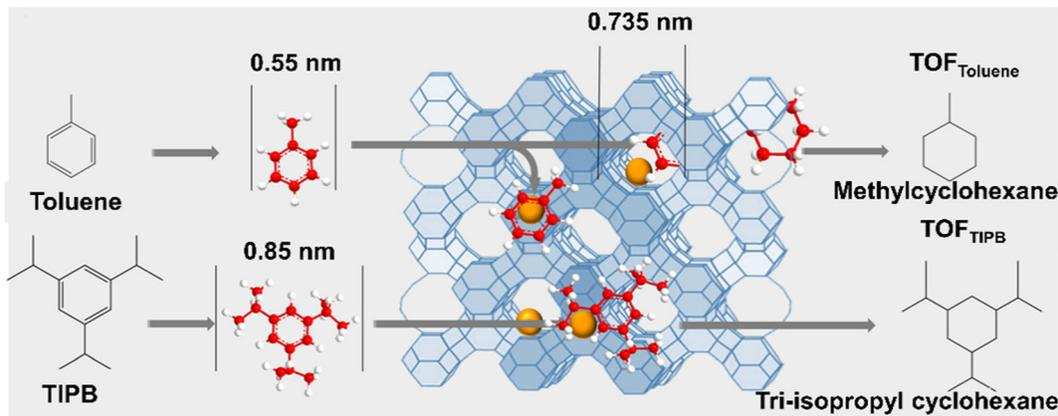
Fig. 12 Diagram of hydrogenation tests with toluene and TIPB as the probing molecules.<sup>107</sup> Reprinted with permission from Wiley-VCH, copyright 2021.
