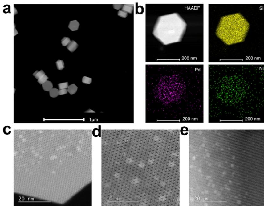
**Fig. 8** (a) STEM and (b) HAADF-STEM image of the 0.8Pd0.2Ni(OH)<sub>2</sub>@S-1 catalyst and the corresponding EDS mapping images for Si, Pd, and Ni elements; (c and d) Cs-corrected HAADF-STEM images of the 0.8Pd0.2Ni(OH)<sub>2</sub>@S-1 catalyst viewed along the *b*-axis orientation with low and high magnification and (e) viewed along other orientation.<sup>45</sup> Reprinted with permission from Elsevier Inc, copyright 2017.
