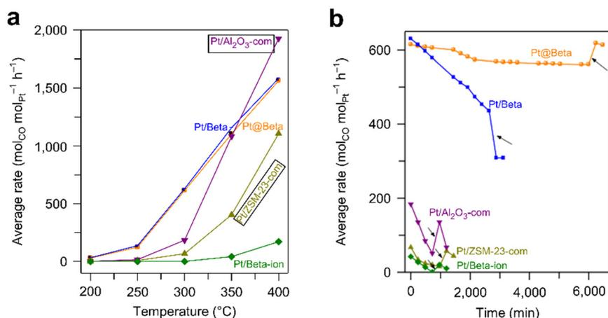
Fig. 18 Average rates of various catalysts in the WGS reaction as a function of (a) temperature and (b) time (reaction conditions: 20 mL min<sup>-1</sup> of reactant gas (7% CH<sub>4</sub> + 3.3% O<sub>2</sub> + 79.7% He), GHSV = 480 000 mL g<sub>Pd</sub><sup>-1</sup> h<sup>-1</sup>, 600 °C).<sup>126</sup> Reprinted with permission from Spring Nature, copyright 2018.
