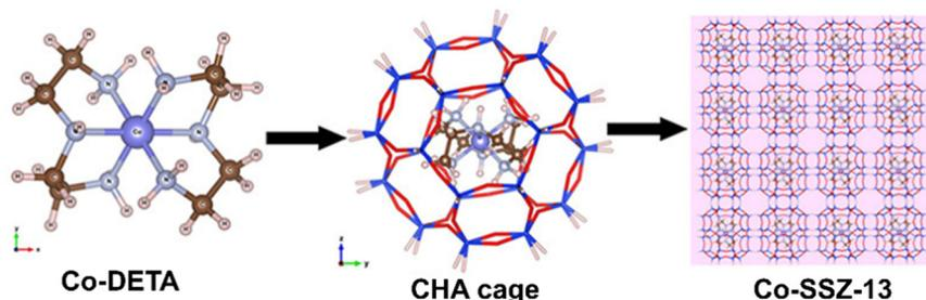
Fig. 6 Positions of Co-DETA complex within the CHA framework.<sup>83</sup> Reprinted with permission from American Chemical Society, copyright 2018.
