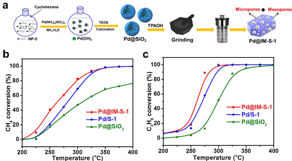
Fig. 13 (a) Schematic diagram of the synthesis of Pd@S-1 catalyst; deep oxidation performance of (b) methane and (c) propane on Pd-based catalysts (reaction conditions: WHSV = 36 000 mL  $g_{cat}^{-1} h^{-1}$ , 0.1 MPa, 200–400 °C).<sup>39</sup> Reprinted with permission from Springer Nature, copyright 2022.
