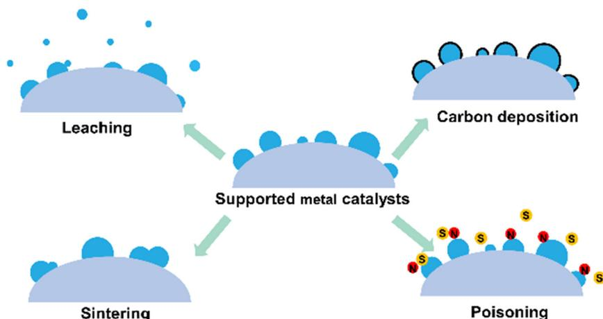
Fig. 17 Schematic of supported metal catalysts deactivation modes.
