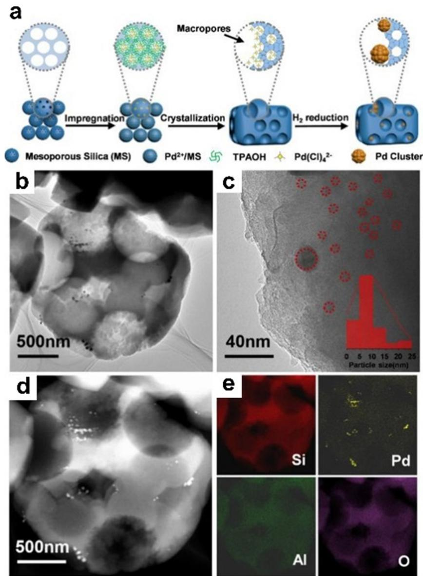
Fig. 20 (a) Synthesis of Pd@ZSM-5; (b and c) TEM images of Pd@ZSM-5; (d) HAADF-STEM image of Pd@ZSM-5, and (e) the corresponding EDS mapping images for Si, Al, Pd, and O elements.<sup>144</sup> Reprinted with permission from Wiley-VCH, copyright 2020.
