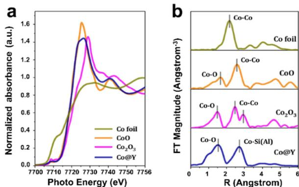
Fig. 9 XAS characterization of the Co@Y sample. (a) Co K-edge XANES spectra; (b) FT  $k^2$ -weighted EXAFS spectra.<sup>101</sup> Reprinted with permission from American Chemical Society, copyright 2022.
