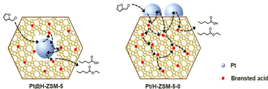
Fig. 16 The conversion of furfural into VA/EV over Pt@H-ZSM-5 and Pt/H-ZSM-5.<sup>27</sup> Reprinted with permission from American Chemical Society, copyright 2020.
