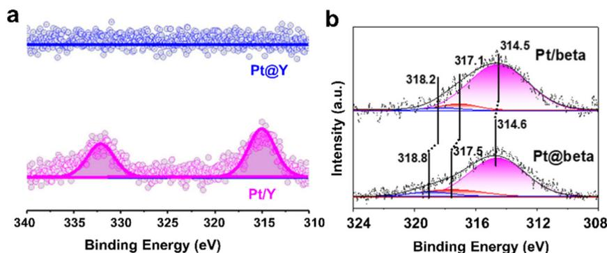
Fig. 10 (a) Pt 4d XPS of Pt@Y and Pt/Y without Ar<sup>+</sup> ion sputtering.<sup>94</sup> Reprinted with permission from American Chemical Society, copyright 2021; (b) Pt 4d XPS of Pt@Beta and Pt/Beta with Ar<sup>+</sup> ion sputtering.<sup>103</sup> Reprinted with permission from Wiley-VCH, copyright 2021.
