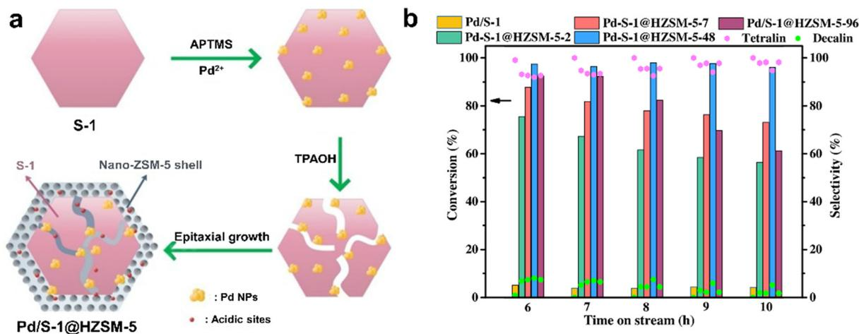
Fig. 14 (a) The preparation progress for the Pd/S-1@HZSM-5 catalyst; (b) catalytic performances of naphthalene hydrogenation over different catalysts (reaction conditions: WHSV = 1.3  $h^{-1}$ ,  $H_2/$ feed = 750, 4 MPa  $H_2$ , 280 °C).<sup>118</sup> Reprinted with permission from Elsevier B.V., copyright 2021.
