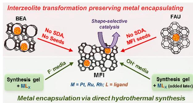
**Fig. 3** Schematic representation of interzeolite transformations progress.<sup>69</sup> Reprinted with permission from American Chemical Society, copyright 2014.
