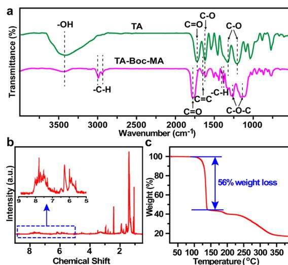
Fig. 1 Structure characterization of TA and the synthesized TA-Boc-MA resin: (a) FTIR spectra of TA and TA-Boc-MA resin; (b) <sup>1</sup>H-NMR spectra of TA-Boc-MA resin in DMSO-*d*<sub>6</sub>; (c) TGA analysis of the TA-Boc-MA resin.
