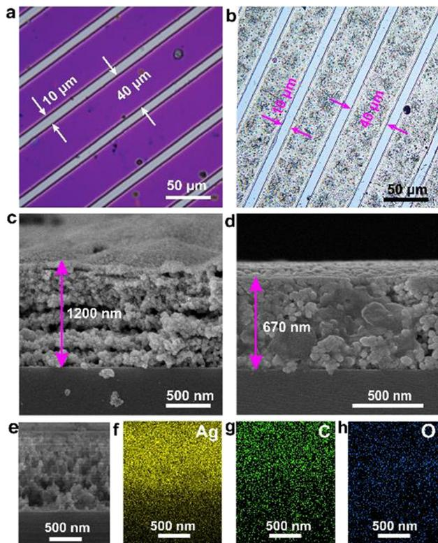
**Fig. 2** Optical images of the lithographic pattern (a) and the corresponding Ag pattern (b) based on the TA-Boc-MA photoresist exposed with a UV light source at 365 nm; cross-sectional SEM images of Ag pattern before (c) and after (d) annealing; cross-sectional SEM image of the Ag pattern (e) and the corresponding EDX mapping images (f–h) before annealing at 200 °C. Electroless deposition time for all the Ag patterns in Fig. 2 is 40 minutes.
