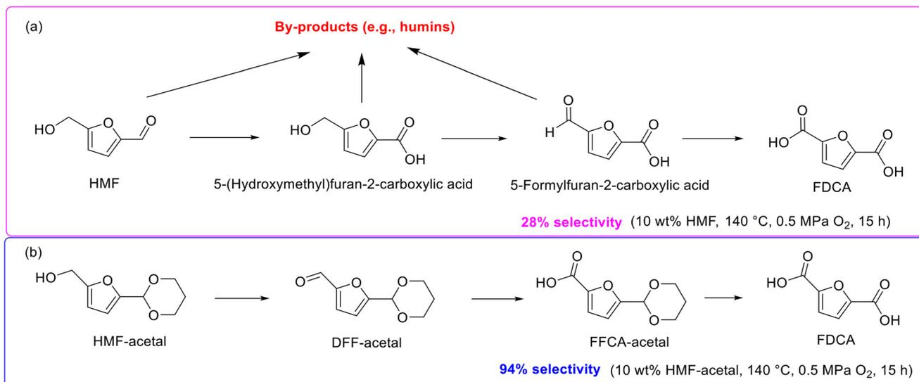
**Scheme 14** Reaction pathways for the synthesis of FDCA from HMF (a) and HMF-acetal (b).
