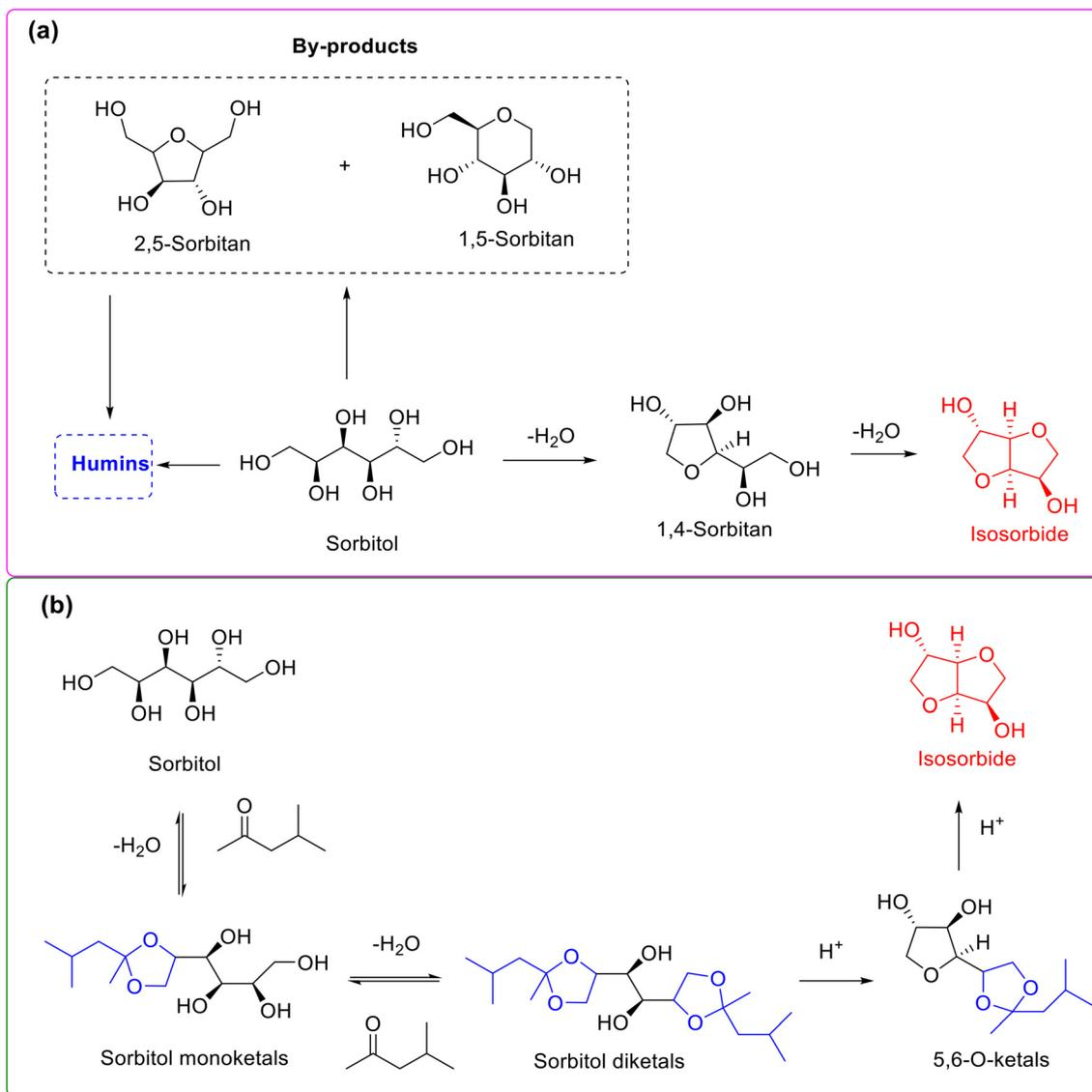
**Scheme 15** Reaction pathway for the synthesis of isosorbide from the dehydration of sorbitol without (a) or with (b) acetalization strategy. Adapted with permission from ref. 165. Copyright 2018, Royal Society of Chemistry.
