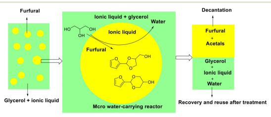
Fig. 4 Schematic showing the acetalization of furfural with glycerol over [BPy]HSO4 ionic liquid in the micro water-removing reactor. Adapted with permission from ref. 92. Copyright 2014, Royal Society of Chemistry.
