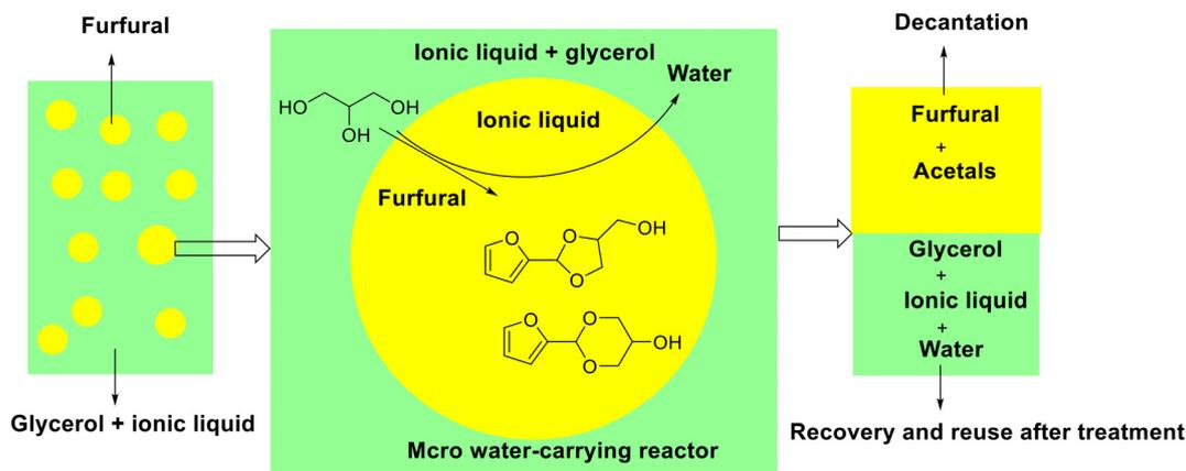
**Fig. 4** Schematic showing the acetalization of furfural with glycerol over [BPy]HSO<sub>4</sub> ionic liquid in the micro water-removing reactor. Adapted with permission from ref. 92. Copyright 2014, Royal Society of Chemistry.
