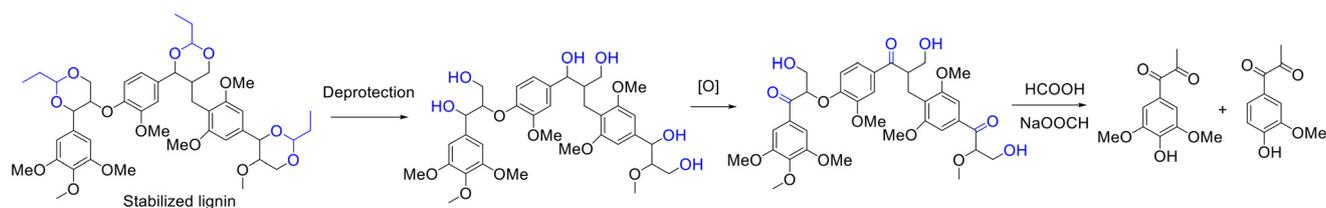
**Scheme 13** Synthesis of syringyl and guaiacyl propane diones from the oxidation of stabilized lignin, followed by depolymerization. Adapted with permission from ref. 155. Copyright 2019, John Wiley and Sons.
