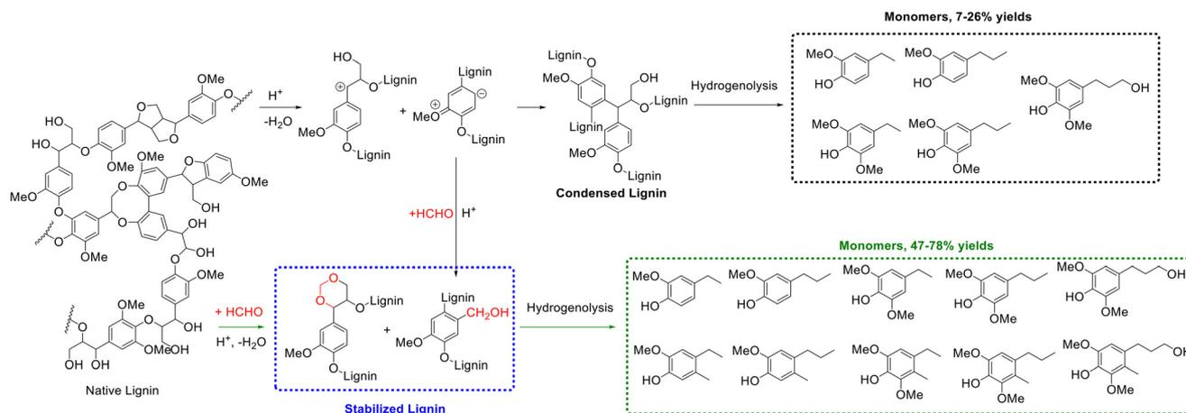
**Scheme 12** Monomers production from extracted lignin (stabilization with formaldehyde or condensed lignin), followed by hydrogenolysis. Adapted with permission from ref. 153. Copyright 2016, American Association for the Advancement of Science.
