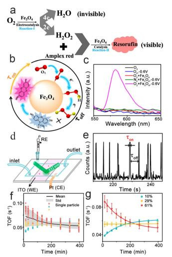
Fig. 7 Reaction mechanism (a) and detection mechanism (b); (c) electrochemically coupled fluorescent light; (d) schematic illustration of a three-electrode microfluidic reaction cell; (e) typical fluorescence burst curve; (f and g) fitting (f) and correlation analysis (g) of kinetic parameters.<sup>81</sup> Reprinted with permission from ref. 81. Copyright 2020, American Chemical Society.
