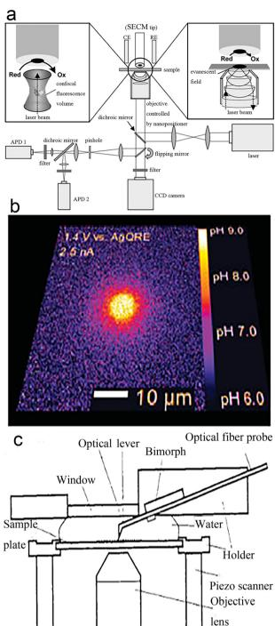
Fig. 12 (a) SECM-TIRFM schematic diagram; (b) a 35 nm-radius nanorode generates a local pH gradient. $^{10\overline{5}}$  Reprinted with permission from ref. 105. Copyright 2004, American Chemical Society. (c) AFM-TIRFM schematic diagram.<sup>111</sup> Reprinted with permission from ref. 111. Copyright 1996, Springer Nature.
