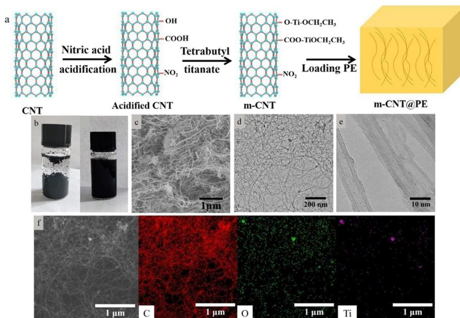
**Fig. 1** (a) Schematic diagram of surface modification steps with CNTs to make PE nanocomposites. (b) Comparison of optical photographs of the original CNTs and m-CNTs in ethanol. (c) SEM and (d and e) TEM images of the m-CNTs. (f) Elemental mapping of the m-CNTs.
