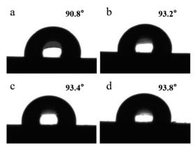
Fig. 9 Surface contact angle of PE and the nanocomposites: (a) PE sample; (b-d) 0.58 wt%, 0.84 wt%, and 1.10 wt% CNT/PE nanocomposites
