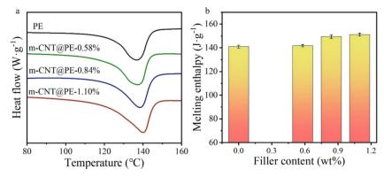
Fig. 4 Comparison of (a) DSC melting curves and (b) enthalpy values of the nanocomposites with increasing m-CNT content.
