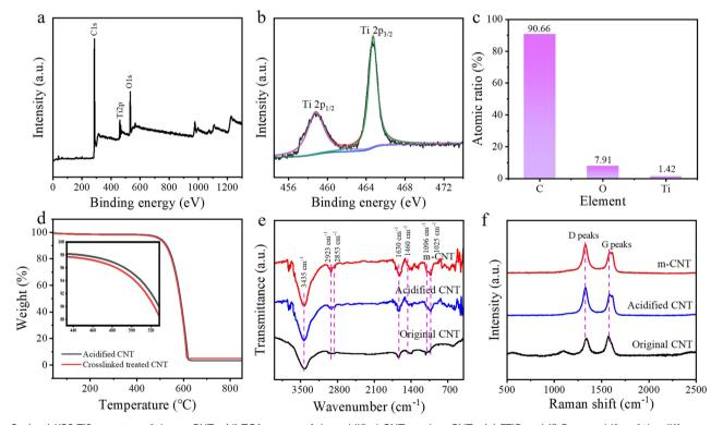
Fig. 2 (a-c) XPS Ti2p spectra of the m-CNTs. (d) TGA curves of the acidified CNTs and m-CNTs. (e) FTIR and (f) Raman shifts of the different CNT samples.
