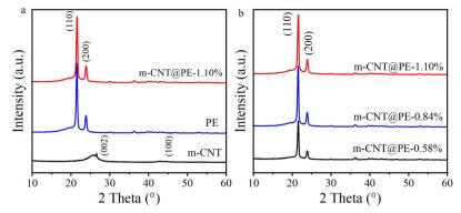
Fig. 3 (a) XRD patterns of the CNT/PE nanocomposite, PE and CNT. (b) XRD patterns of the nanocomposites with increasing CNT content.
