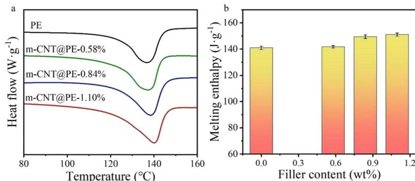
Fig. 4 Comparison of (a) DSC melting curves and (b) enthalpy values of the nanocomposites with increasing m-CNT content.
