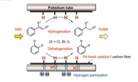
Development of a highly efficient electrocatalytic hydrogenation and dehalogenation system using a flow cell with a Pd tube cathode
