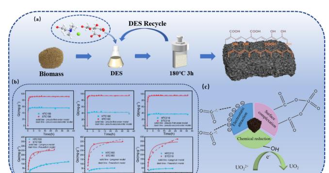
Fig. 9 Synthesis of biocarbons with rich carboxyl and phenol groups *via* DES-mediated HTC for highly efficient uranium adsorption.<sup>10</sup> (a) The scheme for functional biocarbon synthesis *via* DES-mediated HTC. (b) Uranium adsorption kinetics and isotherms for biocarbons from conventional HTC and DES-mediated HTC. (c) Uranium adsorption mechanisms for the resultant biocarbon.
