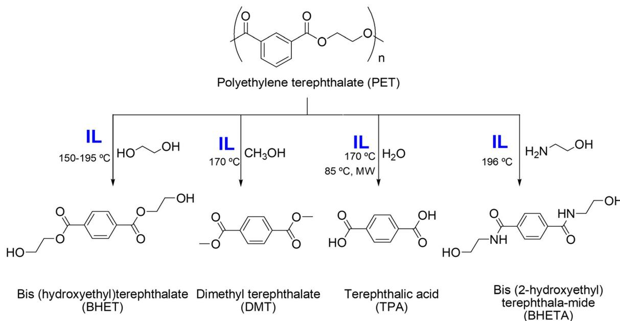
**Fig. 18** Depolymerization of PET to produce terephthalic acid (TPA), dimethyl terephthalate (DMT), bis(hydroxyethyl)terephthalate (BHET), or bis(2-hydroxyethyl)terephthalamide (BHETA), depending on the reaction system, hydrolysis, methanolysis, glycolysis, or aminolysis, respectively, in IL-based media.
