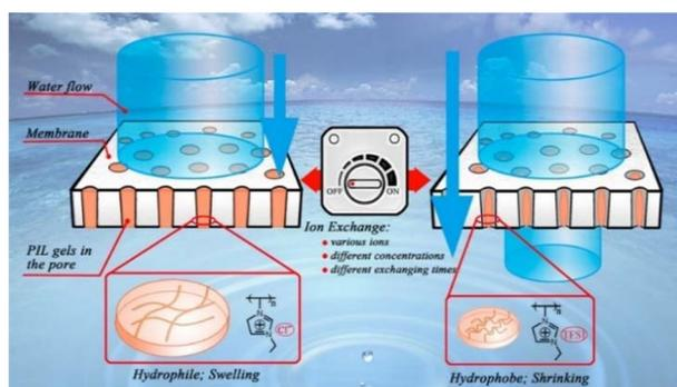
**Fig. 3** Salt-responsive PES membranes integrated with anion-sensitive poly(ionic liquid) (PIL) gels prepared with methacrylateoethyl trimethyl ammonium chloride ([MTA][Cl]). Reproduced from ref. 78 with permission from American Chemical Society, copyright 2017.
