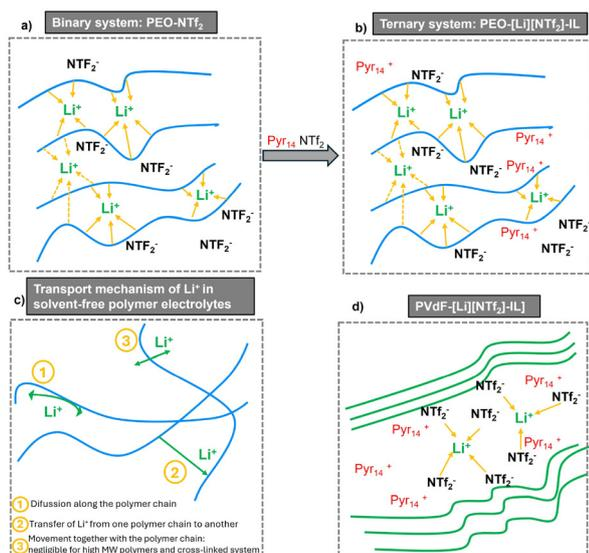
**Fig. 4** (a)  $\text{Li}^+$ -ion coordination and (c) transport mechanisms in PEO-based, binary polymer electrolytes.  $\text{Li}^+$ -ion coordination in ternary polymer electrolytes containing (b) active polymers (e.g. PEO) and (d) inactive polymers (e.g. PVdF). Adapted from ref. 96 with permission from John Wiley & Sons, copyright 2015.
