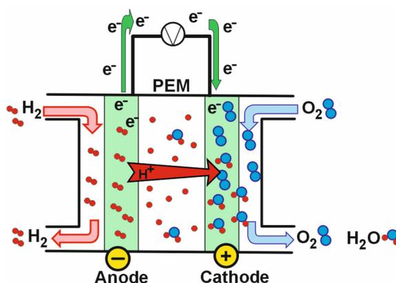
Fig. 6 Schematic representation of a proton exchange membrane fuel cell.<sup>109</sup>
