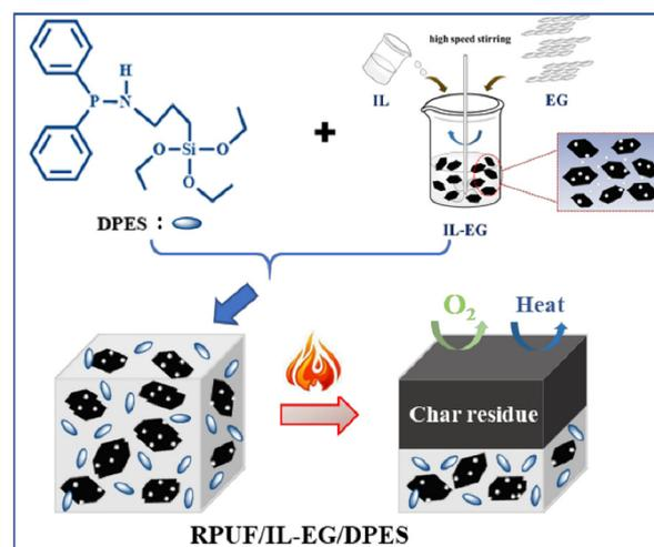
Fig. 7 Schematic representation of the synthesis and burning mechanism of flame-retardant RPUFs compounded with IL-EG/DPES. Reproduced from ref. 117 with permission from Multidisciplinary Digital Publishing Institute, copyright 2020.
