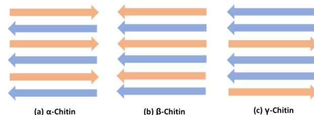
**Fig. 1** Different structural form of chitin (a)  $\alpha$ -chitin, (b)  $\beta$ -chitin, and (c)  $\gamma$ -chitin.<sup>12</sup>
