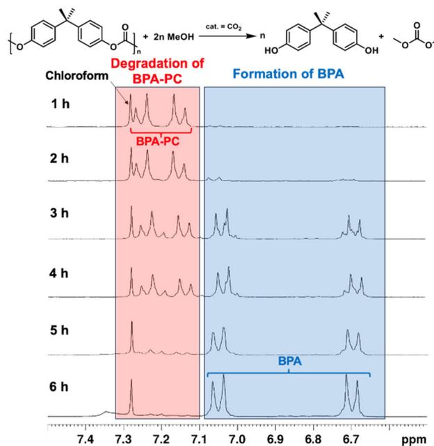
Fig. 4 CO<sub>2</sub> catalyzed methanolysis of the BPA-PC pellets monitored by <sup>1</sup>H NMR spectroscopy (300 MHz, CDCl<sub>3</sub>, 6.5–7.5 ppm). Reaction condition: BPA-PC (508 mg, 2 mmol carbonate units), MeOH (3.2 g, 100 mmol, 50 equivalents relative to carbonate units), CO<sub>2</sub> (1 MPa), T = 140 °C.
