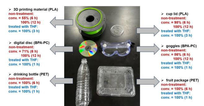
Fig. 6 Depolymerization of end-of-life materials.
