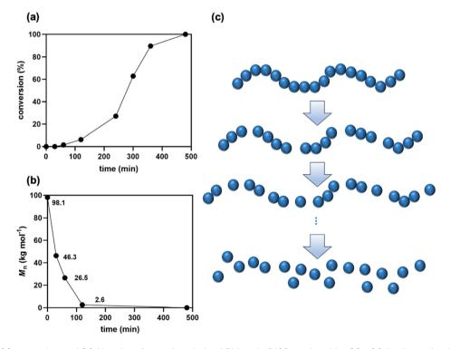
Fig. 3 Changes in (a) conversion and (b) M<sub>n</sub> values for methanolysis of PLA resin R190 catalyzed by CO<sub>2</sub>. (c) A scheme for the depolymerization mode of PLA (random chain scission).
