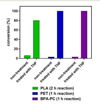
Fig. 5 Comparison of PLA, PET, and BPA-PC methanolysis under non-treatment and pre-treatment in THF conditions.
