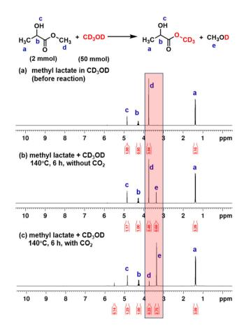
Fig. 1  $\,^{1}$ H NMR spectra of transesterification between methyl lactate and CD $_{3}$ OD.
