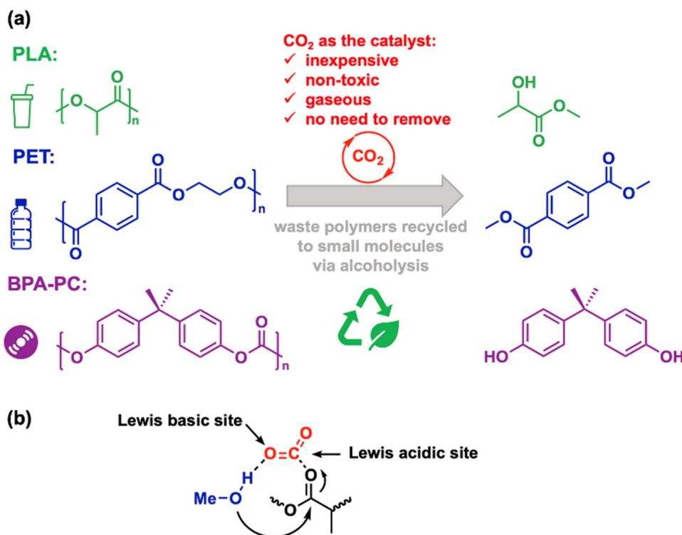
**Scheme 1** (a) CO<sub>2</sub> catalyzed depolymerization and recycling waste polyesters and polycarbonates; (b) CO<sub>2</sub> as a Lewis acid–base pair for activating MeOH and polyester.
