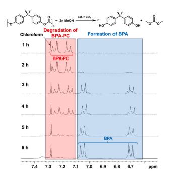
Fig. 4  $CO_2$  catalyzed methanolysis of the BPA-PC pellets monitored by  $^1H$  NMR spectroscopy (300 MHz,  $CDCl_3$ , 6.5–7.5 ppm). Reaction condition: BPA-PC (508 mg, 2 mmol carbonate units), MeOH (3.2 g, 100 mmol, 50 equivalents relative to carbonate units),  $CO_2$  (1 MPa), T = 140.9°C
