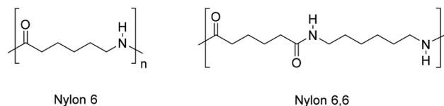
Fig. 11 Structures of nylon 6 and nylon 6,6.
