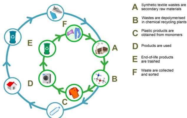
**Fig. 9** Circular economy model based on molecular recycling of synthetic textile waste. A variety of products can be manufactured, including virgin textiles (green loop) or packaging materials (blue loop).
