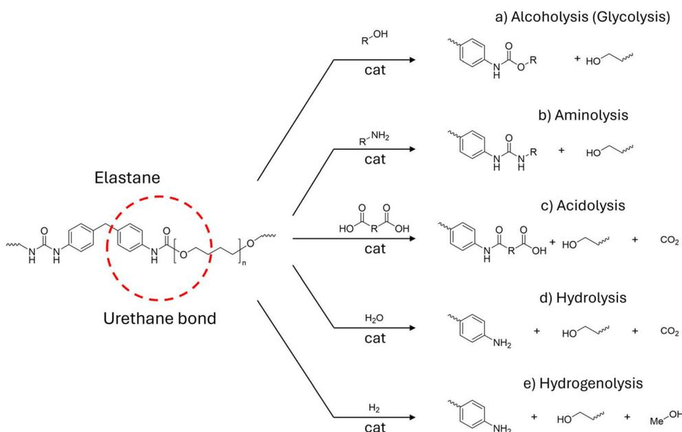
**Fig. 15** Scheme of the major possible EL chemical depolymerization reactions involving the urethane bond using homogeneous-phase catalysts: (a) glycolysis, (b) aminolysis, (c) alcoholysis, (d) hydrolysis, and (e) hydrogenolysis.
