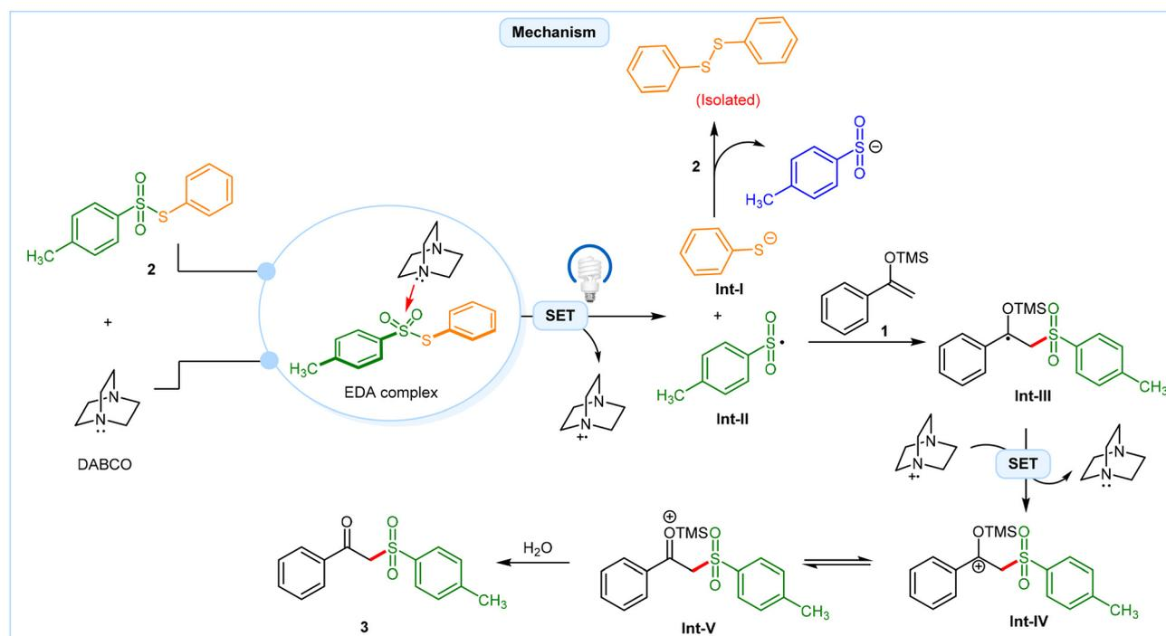
Scheme 3 Possible reaction mechanism.
