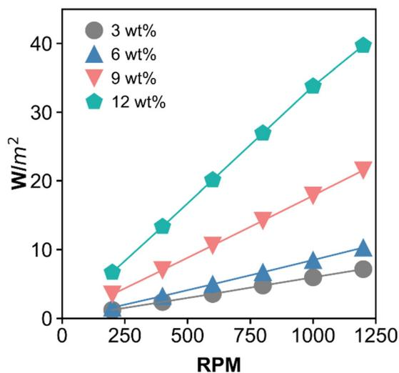
**Fig. 5** The impact of disc rotation velocity and insoluble solids content within the module on the minimum energy demand per square meter of membrane area. The power consumption is calculated from eqn (8)–(10) (see Materials and methods) which then divided the membrane area to derive the energy demand per unit area.
