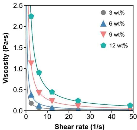
**Fig. 1** The dynamic viscosity of DDR-EH is shown as a function of shear at 3, 6, 9, and 12 wt% insoluble solids. The curve fits are based on eqn (1) using the corresponding power law coefficients and exponent listed in Table 2.
