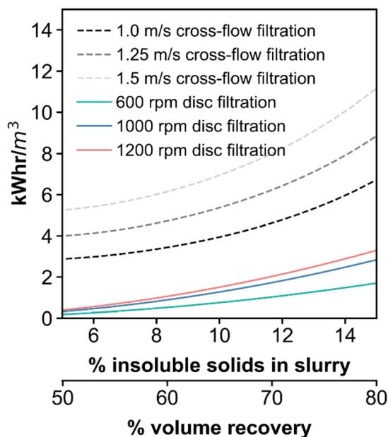
**Fig. 6** Energy consumption on a per volume of permeate calculated for RCD filtration and cross-flow filtration over a range of % insoluble solids in the retentate slurry with the corresponding volume recovery indicated (% feed captured as permeate). Energy demand of cross flow is substantial higher at recommended and demonstrated conditions.
