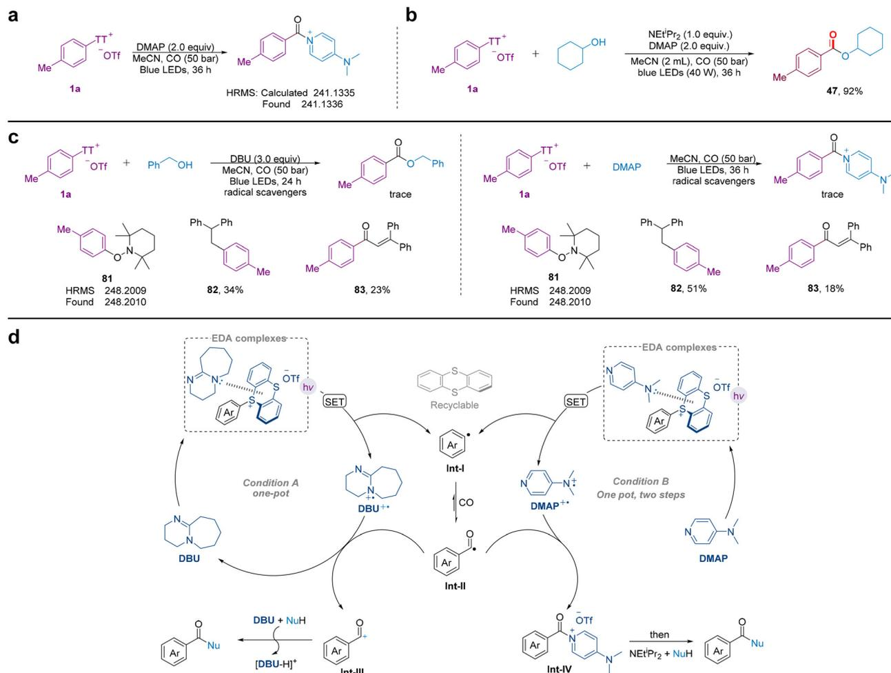
**Fig. 5** Experiments for mechanistic investigation. (a) Detection of the aroyl-DMAP salt. (b) One-pot preparation when DMAP is used as a promoter. (c) Radical-trapping experiment. (d) Possible mechanisms.
