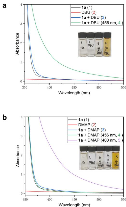
**Fig. 4** Spectroscopic studies of the photochemical carbonylative reaction: (a) UV-vis spectra of **1a** (1) and DBU (2) in MeCN (4 mL) solution and their mixture, taken immediately (3) and after 20 min of irradiation at 456 nm (4); (b) UV-vis spectra of **1a** (1) and DMAP (2) in MeCN (4 mL) solution and their mixture, taken immediately (3) and after 20 min of irradiation at 456 nm (4) and 400 nm (5).
