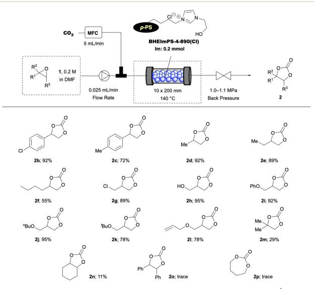
Fig. 4 Substrate scope in continuous-flow cyclic carbonate synthesis. Isolated yields except for 2n, 2o, and 2p (determined by <sup>1</sup>H-NMR analysis).
