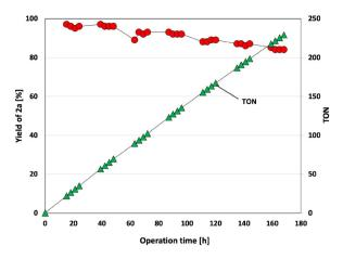
Fig. 5 Extended-time operation for the cycloaddition of 1a and  $CO_2$ . Conditions: 1a, 0.2 M; back pressure, 1.0-1.1 MPa; heater temp., 140 °C; 15.7 mL stainless reactor was utilized. Symbols: red circle, yield of 2a; green triangle, TON based on the amount of imidazolium moiety in the reactor
