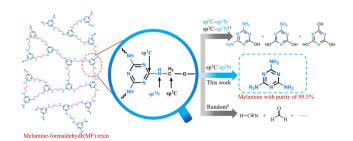
Fig. 1 Structure of MF resin and products formed by the cleavage of different types of chemical bonds.
