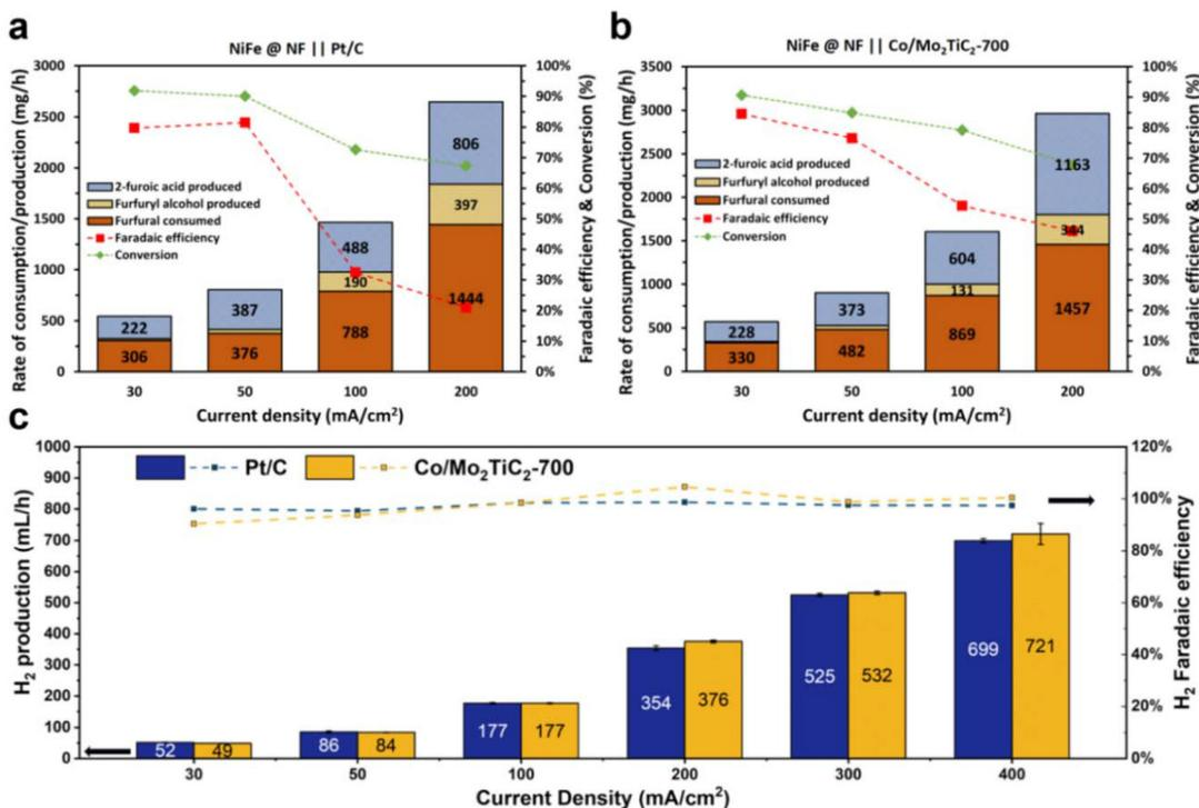
**Fig. 9** Alkaline electrolyzer performance for the cathode and anode. (a) Anode performance when the cathode contains a platinum-based catalyst. (b) Anode performance when the cathode contains a cobalt-based catalyst. (c) Hydrogen production and faradaic efficiency when comparing a cobalt-based catalyst with a platinum-based catalyst.
