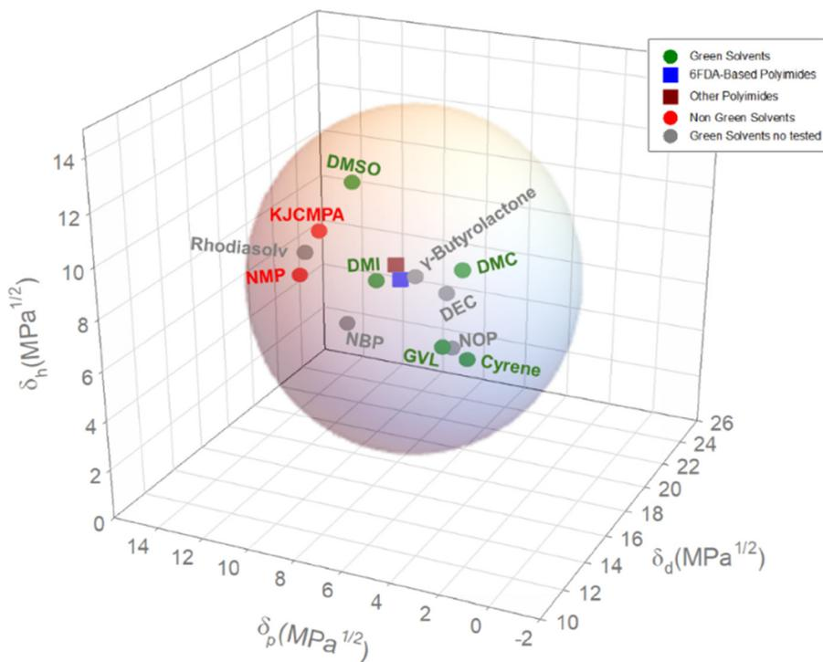
Fig. 4 Three-dimensional Hansen space with axes representing three energy contributions  $\delta_d$ ,  $\delta_p$ , and  $\delta_h$ . The HSP average value for the 6FDA-based polyimides is located at the center of the sphere of radius  $R_0$ .
