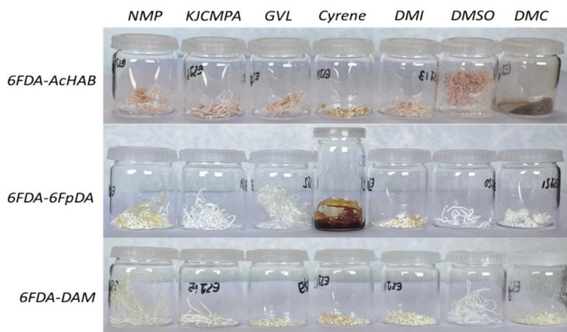
Fig. 5 Polymers 6FDA-AcHAB, 6FDA-6FpDA and 6FDA-DAM synthesized in that order in NMP, KJCMIPA, GVL, Cyrene™, DMI, DMSO, and DMC.
