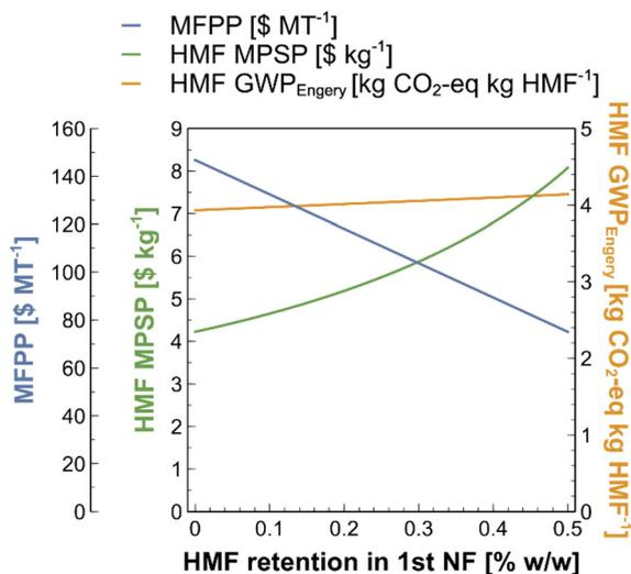
Fig. 6 MFPP, HMF MPSP and HMF GWP<sub>100</sub> using energy allocation at different HMF retention in 1st NF (nanofiltration) using baseline assumptions of other parameters.
