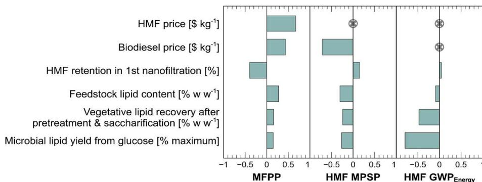
**Fig. 3** Spearman's  $\rho$  values between parameters and MFPP, HMF MPSP, and energy-allocated HMF GWP<sub>100</sub>.
