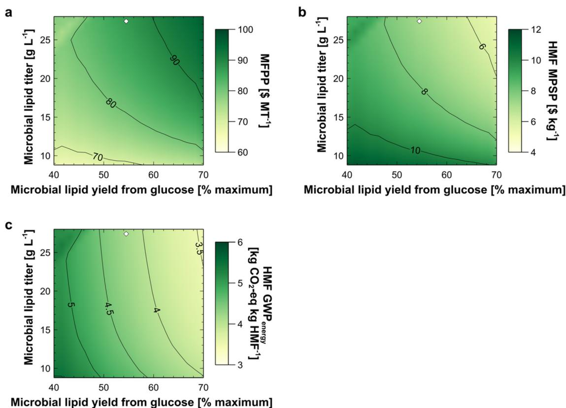
Fig. 4 (a) MFPP, (b) HMF MPSP and (c) HMF GWP<sub>100</sub> using energy allocation at different combinations of microbial lipid yield from glucose and microbial lipid titer using baseline assumptions of other parameters. Diamond markers represent values obtained from the baseline biorefinery.
