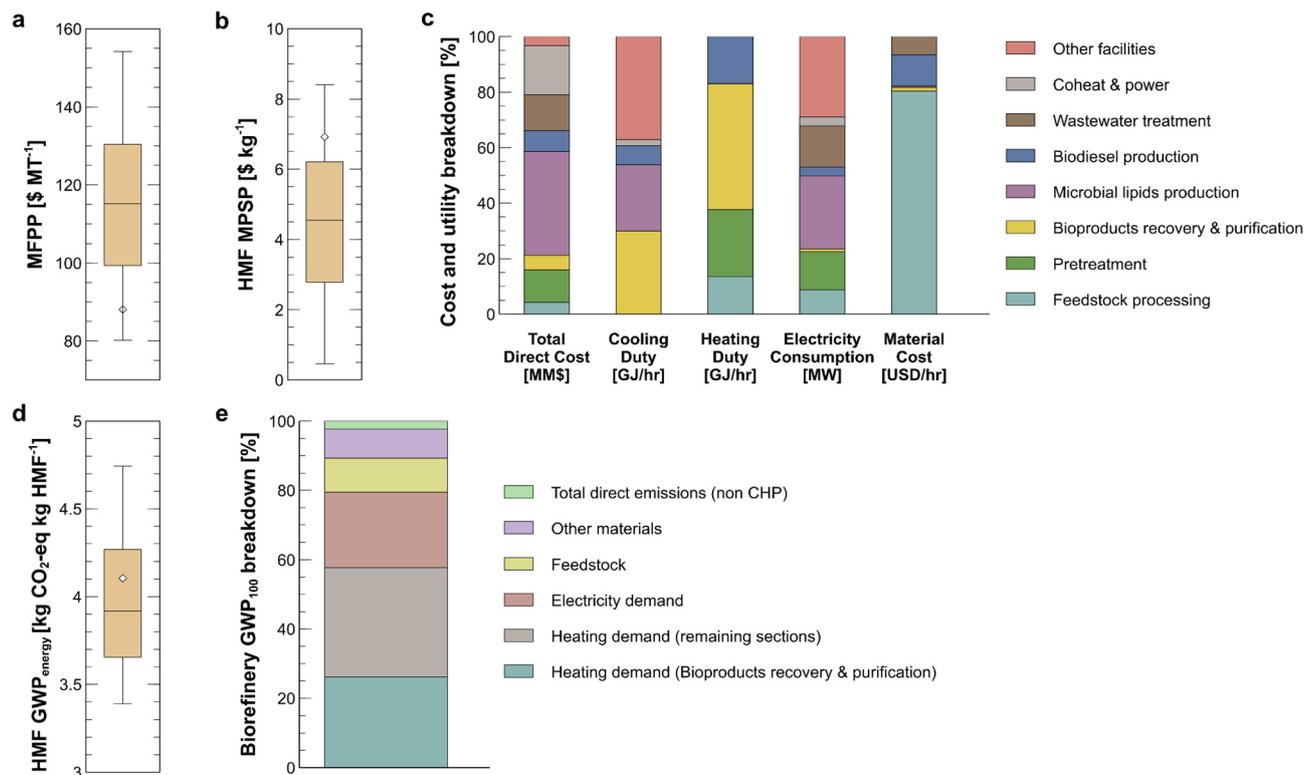
**Fig. 2** Cost estimation and environmental impacts of the biorefinery. Box and whisker plots of (a) MFPP and (b) HMF MPSP, (c) breakdown of total direct cost and utility usage of baseline biorefinery, (d) box whisker plot and (e) breakdown of HMF GWP<sub>100</sub>. Diamond markers in box and whisker plots represent values obtained from baseline biorefinery.
