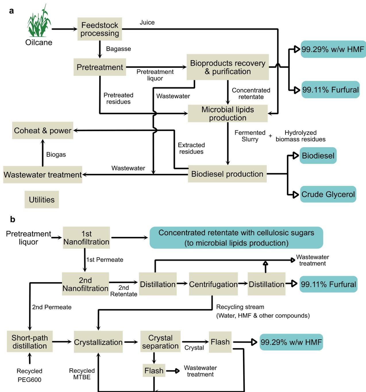
**Fig. 1** Simplified flow diagram of the proposed biorefinery for (a) coproduction of HMF, furfural, biodiesel, and crude glycerol from oilcane, and (b) bioproducts recovery and purification section of the proposed biorefinery. Acronyms in the figure denote polyethylene glycol 600 (PEG600), and methyl *tert*-butyl ether (MTBE).
