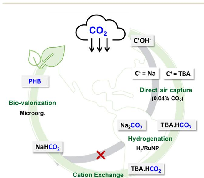
Fig. 6 Schematic representation of a pipeline for atmospheric CO<sub>2</sub> capture and transformation in biodegradable polymers.
