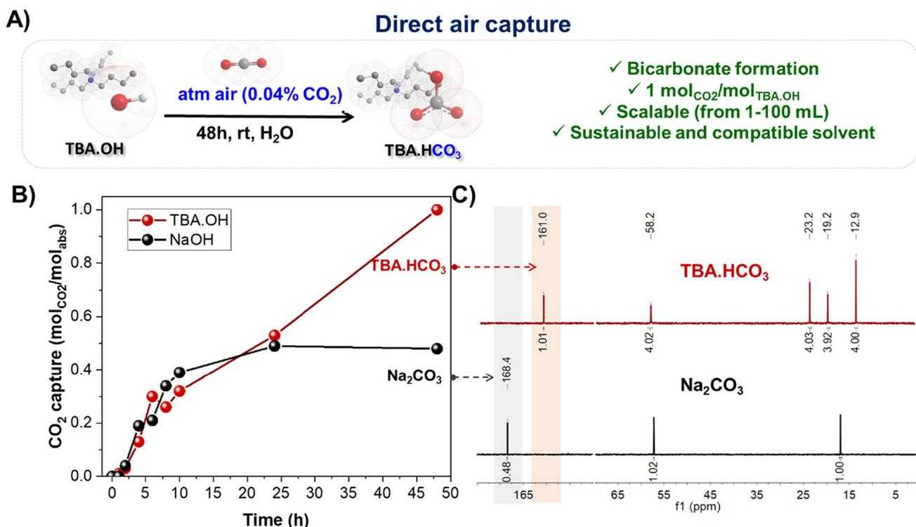
Fig. 2 DAC methodology. (A) General scheme of CO<sub>2</sub> capture. Cations are not represented at scale for clarity. (B) Sorption capacity with different hydroxide salts (sorption conditions: 10 mL of hydroxide solution, 1 mol L<sup>-1</sup> in H<sub>2</sub>O, bubbling compressed air (75 mL min<sup>-1</sup>), 25 °C, 48 h). (C) Quantitative <sup>13</sup>C NMR analysis of captured solutions (Na<sub>2</sub>CO<sub>3</sub> using ethanol as the internal standard).
