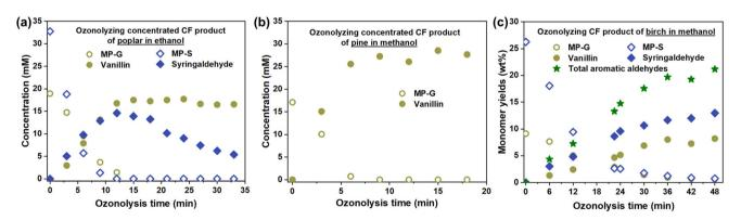
Fig. 4 Ozonolysis of CF products of (a) poplar, (b) pine, and (c) birch. The CF products and conditions are exhibited in Fig. S2.† Ozonolysis conditions: for (a) and (b), 30 mL of concentrated substrate solution or (c) all liquid CF product, and 300 mL min<sup>-1</sup> O<sub>3</sub>/O<sub>2</sub> gas flow at a O<sub>3</sub> concentration of 60 (30 for (c)) mg  $L^{-1}$ . Detailed procedures can be found in ESI S2.3.†
