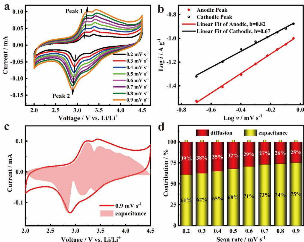
Fig. 7 (a) CV curves at different scanning rates; (b) the fitted  $b$  values determined by the peak current and scanning rate; (c) schematic diagram of the capacitive contribution at  $0.9 \text{ mV s}^{-1}$ ; and (d) capacity contribution ratio at various scanning rates of  $\text{FeF}_3\text{@NPC}$ .
