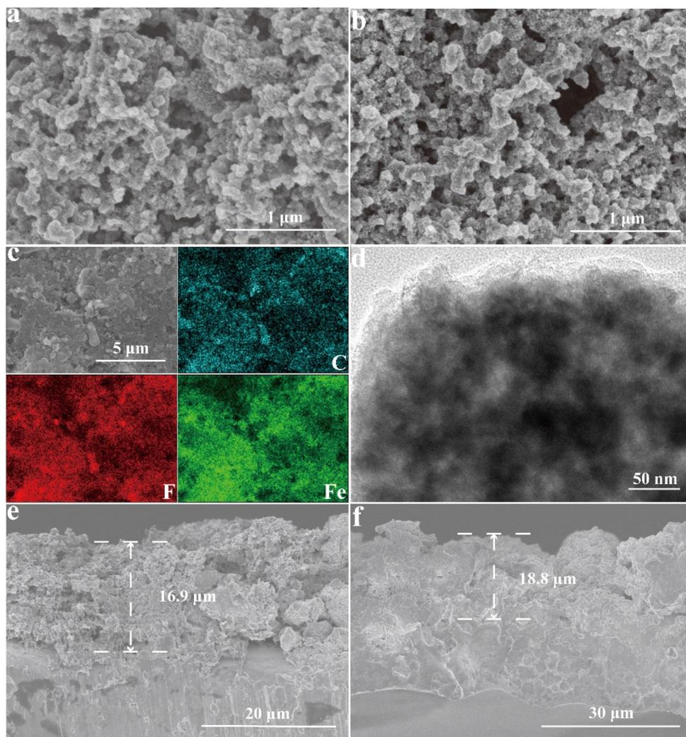
**Fig. 6** (a and b) SEM images of the  $\text{FeF}_3$ @NPC cathode before and after 100 cycles. (c) EDS elemental mappings, and (d) TEM image of the  $\text{FeF}_3$ @NPC cathode after 100 cycles. (e and f) Cross-sectional SEM images of the  $\text{FeF}_3$ @NPC cathode before and after 100 cycles.
