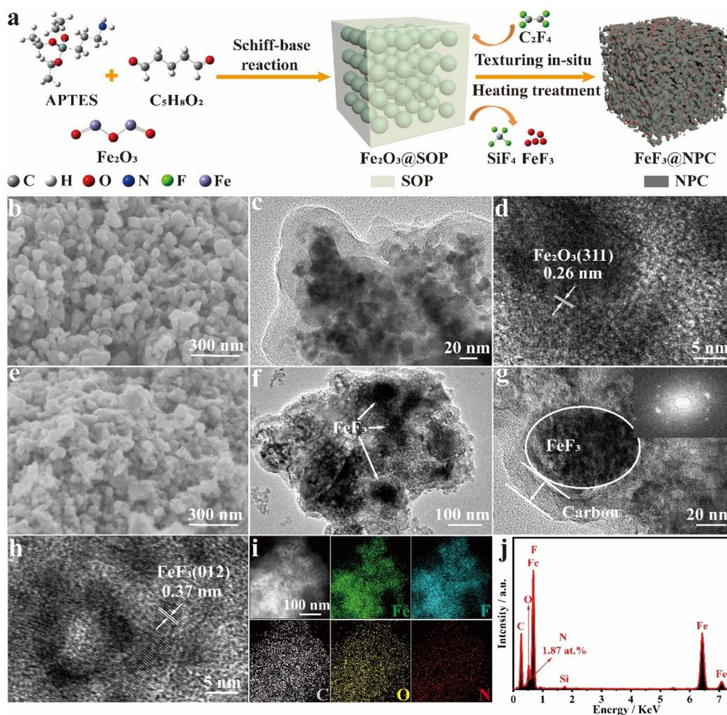
**Fig. 1** (a) Schematic illustration of  $\text{FeF}_3$ @NPC synthesis. (b) SEM, (c) TEM, and (d) HRTEM images of  $\text{Fe}_2\text{O}_3$ @SOP. (e) SEM image, (f and g) TEM images, (h) HRTEM image, (i) STEM and corresponding elemental mappings, and (j) EDX spectrum of  $\text{FeF}_3$ @NPC.
