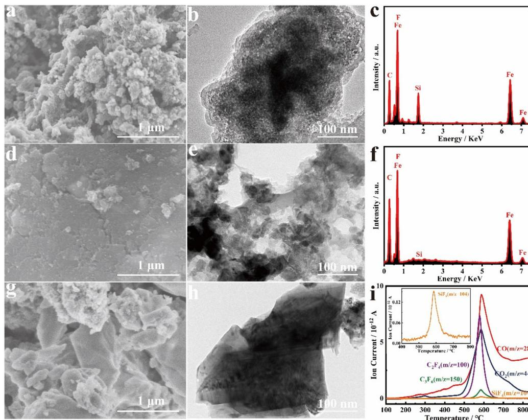
**Fig. 3** (a) SEM image, (b) TEM image, and (c) EDX spectrum of the product obtained by the mass ratio of PTFE/ $\text{Fe}_2\text{O}_3\text{@SOP}$  = 3:1. (d) SEM image, (e) TEM image, and (f) EDX spectrum of the product obtained by the mass ratio of PTFE/ $\text{Fe}_2\text{O}_3\text{@SOP}$  = 10:1. (g) SEM image, and (h) TEM image of the product obtained under 800 °C. (i) Gas emission curves of PTFE and  $\text{Fe}_2\text{O}_3\text{@SOP}$  mixture during the pyrolysis process.
