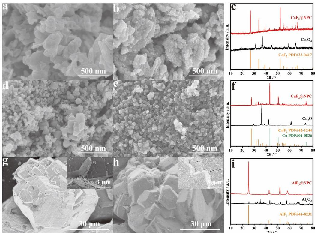
**Fig. 4** (a) SEM image of  $\text{Co}_3\text{O}_4$ , (b) SEM image, and (c) XRD patterns of  $\text{CoF}_2@NPC$ . (d) SEM image of  $\text{Cu}_2\text{O}$ , (e) SEM image, and (f) XRD patterns of  $\text{CuF}_2@NPC$ . (g) SEM image of  $\text{Al}_2\text{O}_3$ . (h) SEM image and (i) XRD patterns of  $\text{AlF}_3@NPC$ .
