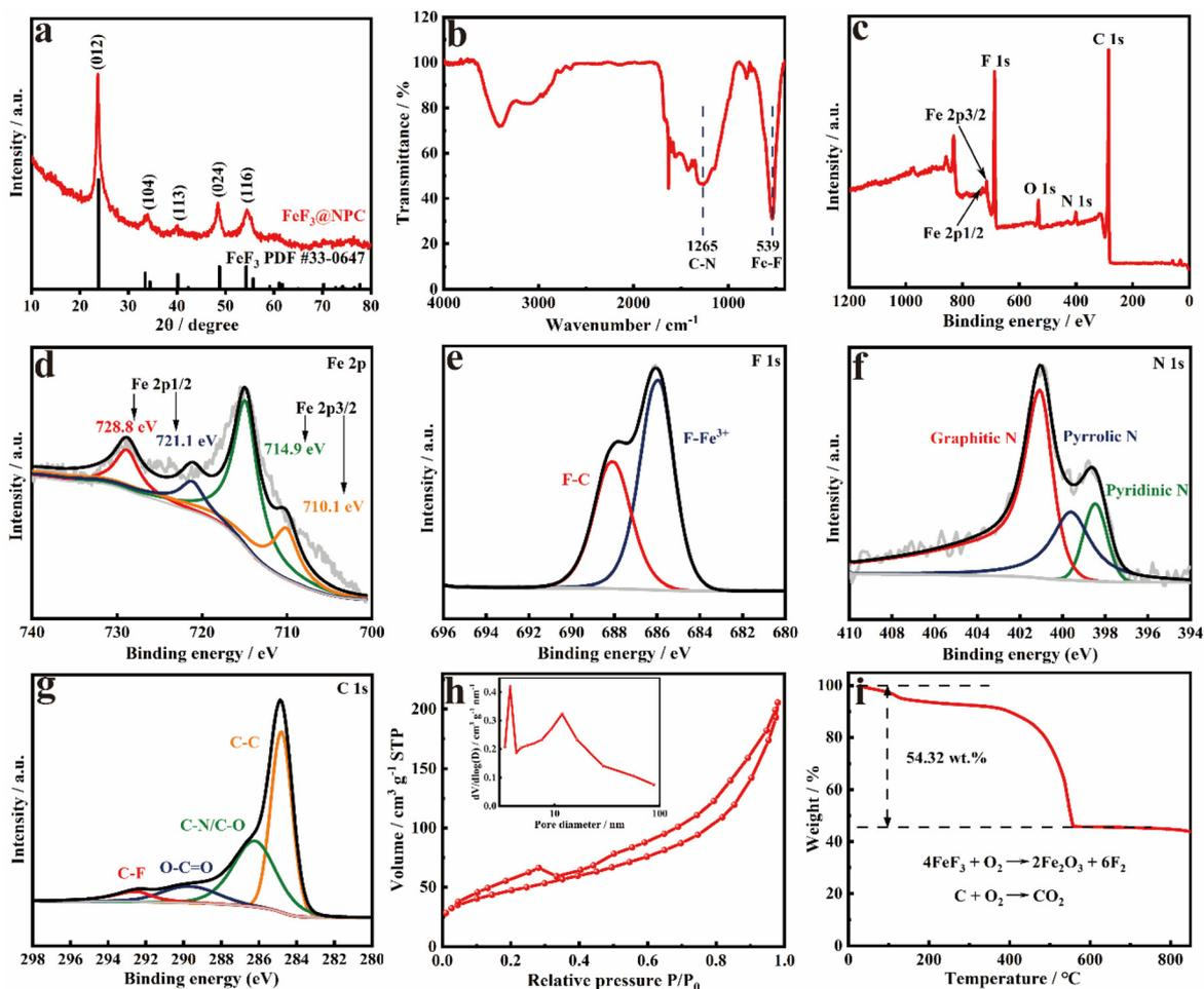
Fig. 2 (a) XRD patterns, (b) FTIR spectra, (c) XPS survey spectrum, (d) Fe 2p, (e) F 1s, (f) N 1s and (g) C 1s XPS spectra, (h) N<sub>2</sub> sorption isotherm and pore size distribution, and (i) TGA curve in air of FeF<sub>3</sub>@NPC.
