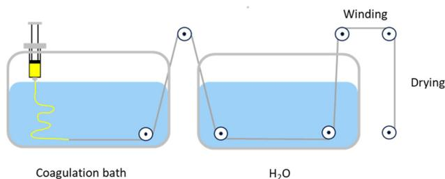
Fig. 5 Double-diffusion wet spinning apparatus used to form cellulose fibres. Adapted from Li *et al.*<sup>49</sup> with permission from American Chemical Society, 2024.
