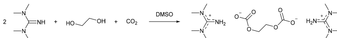
Scheme 4 The formation of a guanidinium ethylene di-carbonate used for non-derivative cellulose dissolution. 41
