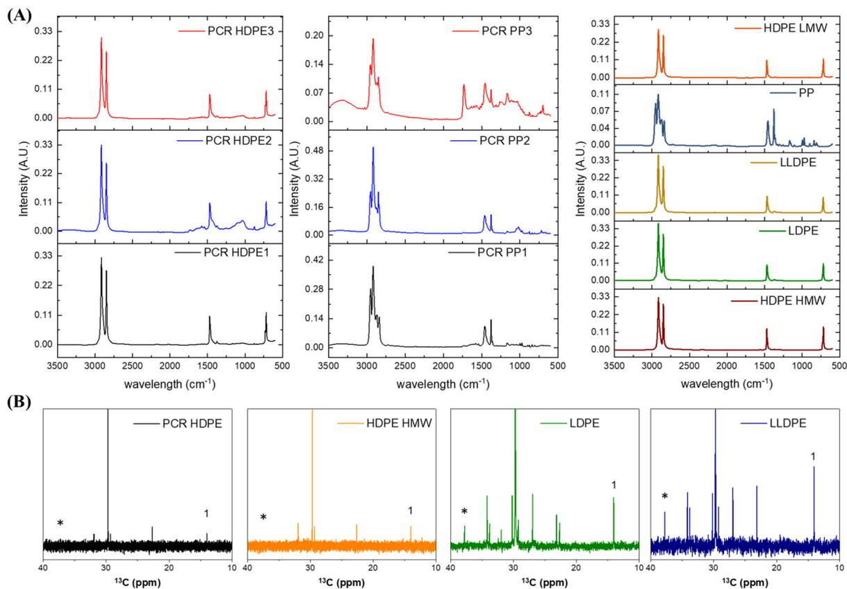
**Fig. 1** (A) ATR-FTIR spectra of PCR HDPE, PCR PP and virgin polyolefins used in this study. (B) Zoomed-in quantitative <sup>13</sup>C NMR results for PCR HDPE, HDPE HMW, LDPE, and LLDPE. The \* symbol is the tertiary carbon and 1 refers to the primary carbon, which indicates the end groups.
