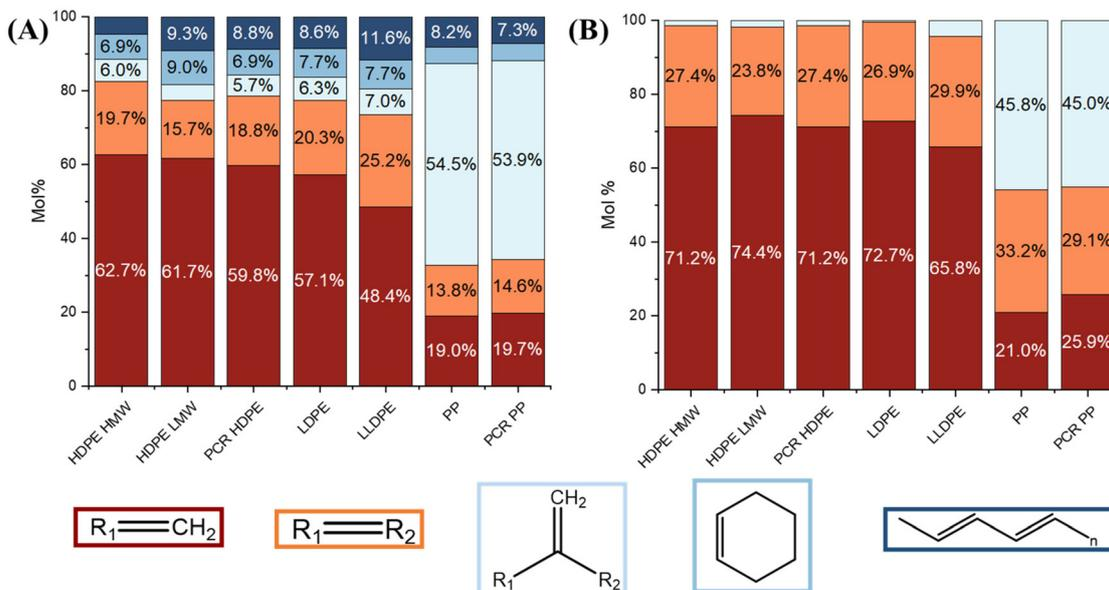
Fig. 5 Normalized molar percentage of terminal (crimson), internal (orange), 1,1-disubstituted (light blue), and cyclic (mid-blue) alkenes, as well as conjugated dienes (navy blue) quantified through <sup>1</sup>H NMR for (A) light oils and (B) heavy oils.
