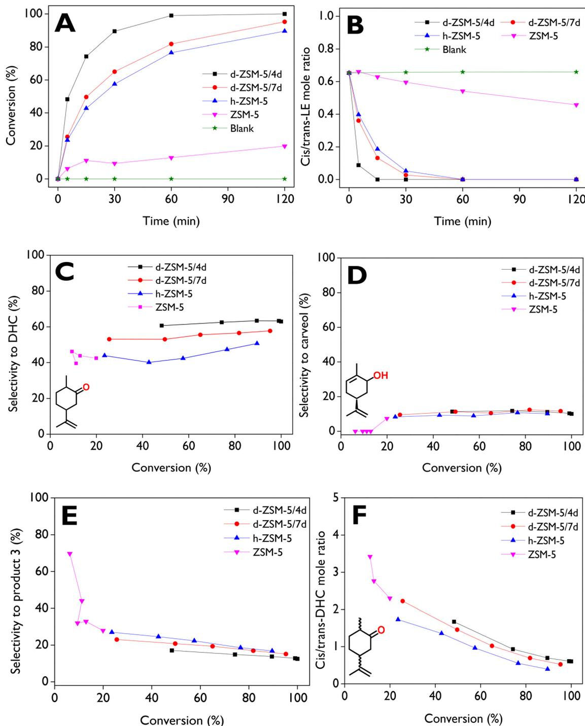
**Fig. 5** (A) Limonene-1,2-epoxide conversion and (B) *cis/trans* limonene-1,2-epoxide molar ratio as a function of the reaction time, (C) selectivity to dihydrocarvone, (D) selectivity to carveol, (E) selectivity to product **3**, and (F) *cis/trans* dihydrocarvone molar ratio, as a function of the conversion. Reaction conditions:  $C_{LE,0} = 13 \text{ mmol L}^{-1}$ , 75 mL of total volume, anhydrous ethyl acetate as a solvent, 115 mg of catalyst, 70 °C, 520–530 rpm,  $N_2$  atmosphere.
