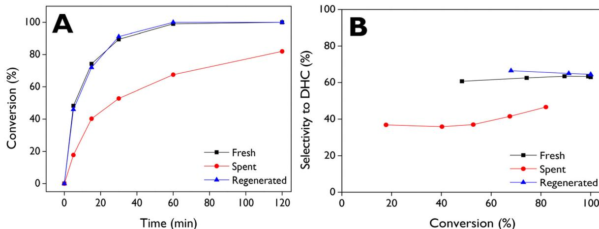
**Fig. 8** Reusability of d-ZSM-5/4d on the LE isomerization. (A) LE conversion as a function of reaction time and (B) selectivity to dihydrocarvone as a function of the conversion. Reaction conditions:  $C_{LE,0} = 13 \text{ mmol L}^{-1}$ , 75 mL of total volume, anhydrous ethyl acetate as a solvent, 115 mg of catalyst, 70 °C, 520–530 rpm,  $N_2$  atmosphere.
