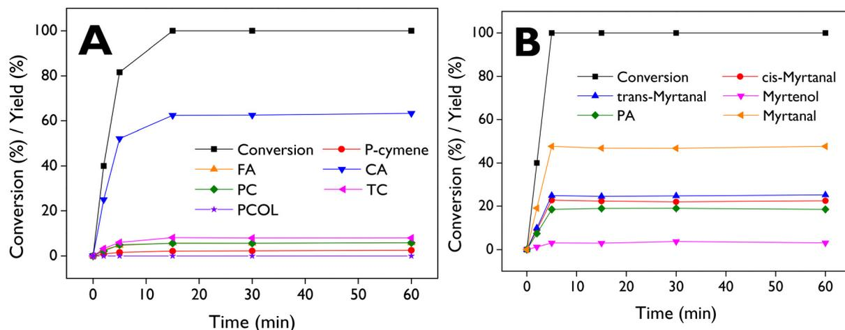
**Fig. 9** Conversion and product distribution of the isomerization of (A)  $\alpha$ -pinene epoxide (60 °C) and (B)  $\beta$ -pinene epoxide (50 °C) over d-ZSM-5/4d. FA: fencholenic aldehyde, CA: campholenic aldehyde, PC: pinocamphone, TC: *trans*-carveol, PCOL: pinocarveol, PA: perillyl alcohol. Reaction conditions:  $C_0 = 13 \text{ mmol L}^{-1}$ , 75 mL of total volume, anhydrous ethyl acetate as a solvent, 115 mg of catalyst, 520–530 rpm,  $N_2$  atmosphere.
