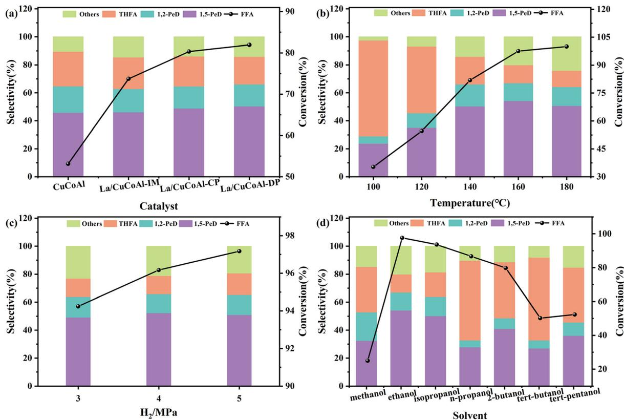
**Fig. 3** The test for the hydrogenation of FFA. (a) Effect of catalyst, (b) Effect of temperature, (c) Effect of H<sub>2</sub> pressure, (d) Effect of solvent. Reaction conditions: FFA 0.5 g, catalyst 0.1 g, ethanol 39.5 g, reaction time 2 h, carbon balance in all reactions  $\geq 97\%$ . THFA: tetrahydrofurfuryl alcohol; FFA: furfuryl alcohol; 1,2-PeD: 1,2-pentanediol; 1,5-PeD: 1,5-pentanediol, others: *n*-pentanol, 2-pentanol and 1-butanol, 2-MF: 2-methylfuran.
