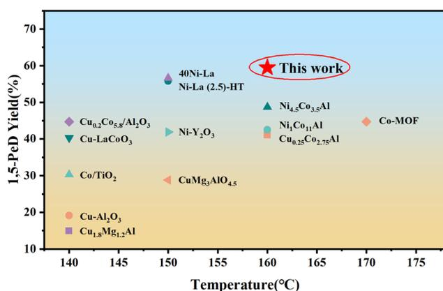
**Fig. 12** The comparison of the catalytic ability of La/CuCoAl-DP with the non-noble metal catalysts reported in the literature (refer to Table S9<sup>†</sup> for details).
