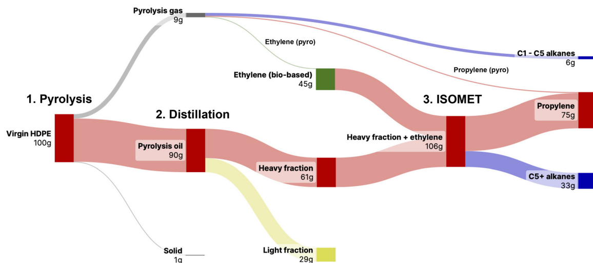
Fig. 5 Total mass balances of the HDPE polymer pretreatment and ISOMET process. The complete olefin ISOMET conversion of the heavy fraction was demonstrated on post-consumer HDPE pyrolysis oil. The remaining alkanes can be further utilized by pyrolysis or catalytic dehydrogenation.
