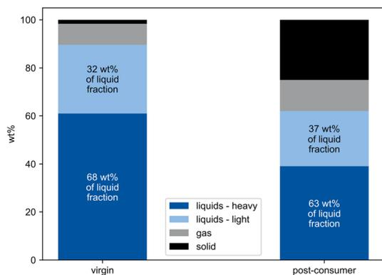
**Fig. 2** Top: conversion of assorted post-consumer HDPE plastic waste to pyrolysis oil. The post-consumer HDPE was initially shredded (1) and then subjected to slow pyrolysis (2) resulting in pyrolysis oils (see ESI† for further information). Bottom: composition of pyrolysis products of virgin and post-consumer HDPE.
