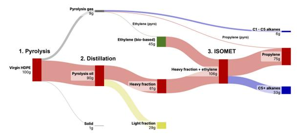
Fig. 5 Total mass balances of the HDPE polymer pretreatment and ISOMET process. The complete olefin ISOMET conversion of the heavy fraction was demonstrated on post-consumer HDPE pyrosis oil. The remaining alkanes can be further utilized by pyrolysis or catalytic dehydrogenation.
