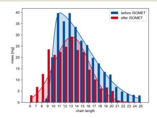
Fig. 3 Analysis of communal heavy pyrolysis oil at appr. 30% olefin conversion. Composition before (blue) and after (red) the ISOMET reaction. ISOMET conditions:  $n(2) = 4.1 \mu mol$ ,  $n(RuH) = 105 \mu mol$ ,  $m(pyrolysis oil) = 0.8 g, V(toluene) = 5.5 mL, <math>p_{ethylene} = 10 \text{ bar}$ ,  $T = 75 \, ^{\circ}\text{C}$ , t = 24 h. (See ESI†).
