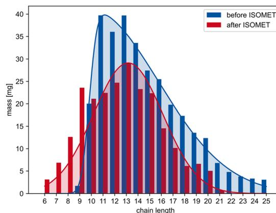
**Fig. 3** Analysis of communal heavy pyrolysis oil at appr. 30% olefin conversion. Composition before (blue) and after (red) the ISOMET reaction. ISOMET conditions:  $n(2) = 4.1$   $\mu\text{mol}$ ,  $n(\text{RuH}) = 105$   $\mu\text{mol}$ ,  $m(\text{pyrolysis oil}) = 0.8$  g,  $V(\text{toluene}) = 5.5$  mL,  $p_{\text{ethylene}} = 10$  bar,  $T = 75^\circ\text{C}$ ,  $t = 24$  h. (See ESI†).
