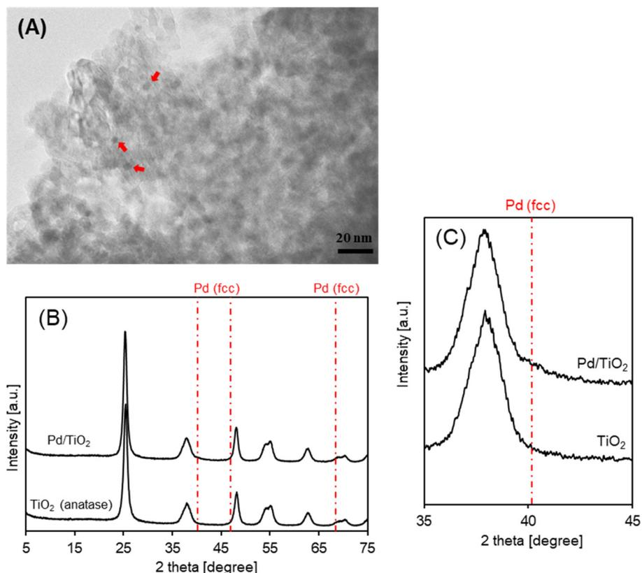
**Fig. 4** Characterization data of the Pd/TiO<sub>2</sub> catalyst (Pd = 3 wt%, *D* = 24%). (A) TEM image, (B) XRD pattern, and (C) XRD pattern around the Pd peak. Conditions: measured after liquid phase reduction at 373 K in water and drying at 383 K in air.
