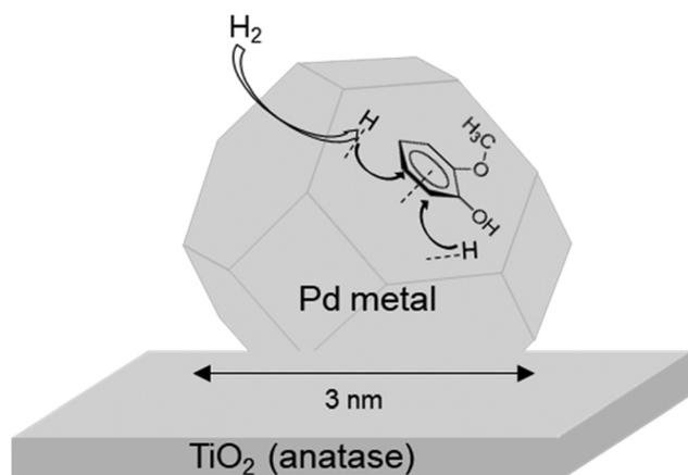
**Fig. 5** Plausible active site of the Pd/TiO<sub>2</sub> catalyst for the selective hydrogenation of guaiacol.
