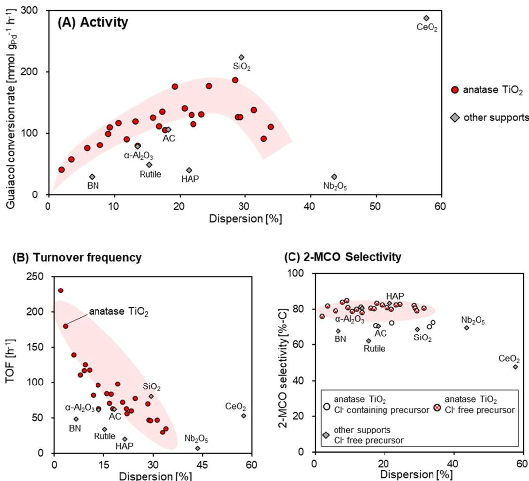
**Fig. 2** Correlation between Pd dispersion and the catalytic activity of selective hydrogenation of guaiacol over supported Pd catalysts. (A) Guaiacol conversion rate, (B) turnover frequency, and (C) 2-MCO selectivity. Conditions: guaiacol (0.62 g), catalyst (100 mg), water (10 g), 373 K, H<sub>2</sub> (1 MPa at r.t.). Dispersion (%) =  $\left[ \frac{\text{amount(mol) of adsorbed CO}}{\text{total amount(mol) of Pd}} \right] \times 100$ .
