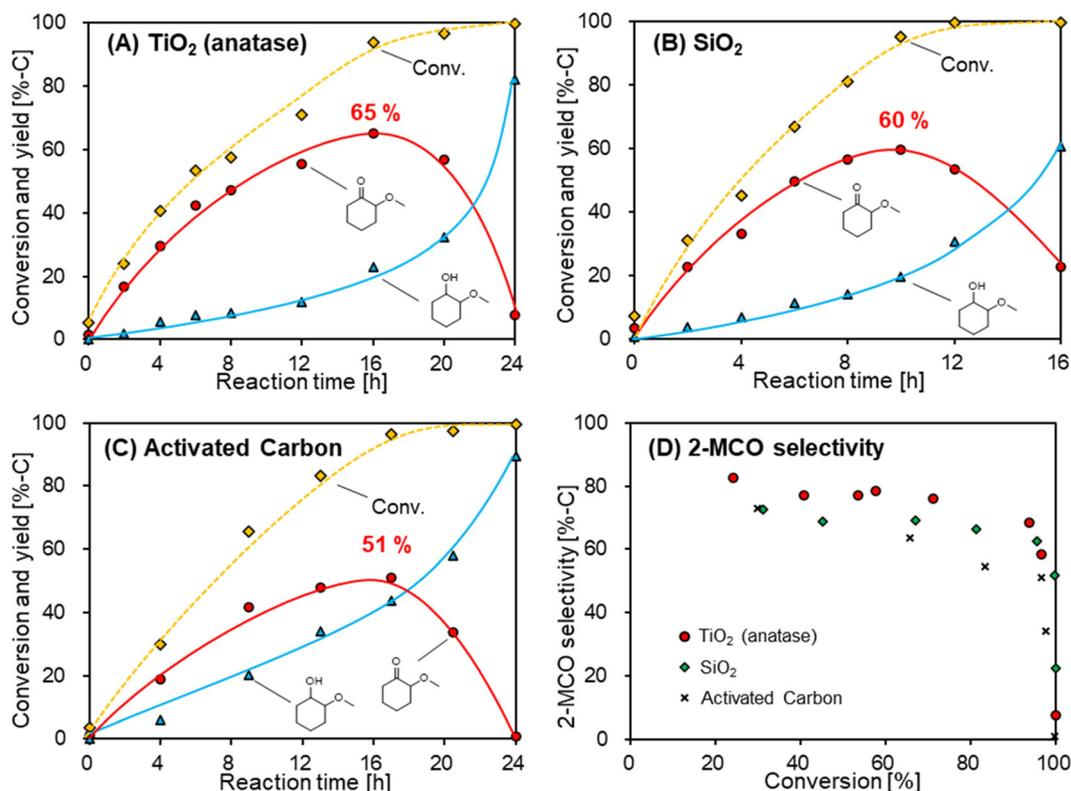
**Fig. 1** Time courses of selective hydrogenation of guaiacol over Pd catalysts on various supports. Conditions: guaiacol (0.62 g), catalyst (Pd = 3 wt%, 100 mg), water (10 g), 373 K, H<sub>2</sub> (1 MPa at r.t.). (A): Anatase TiO<sub>2</sub> support, (B) SiO<sub>2</sub> support, (C) activated carbon support, and (D) selectivity of 2-MCO.
