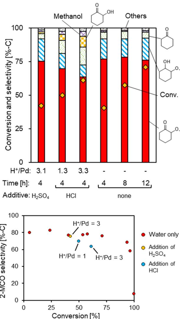
**Fig. 3** Effect of chloride ions on the selective hydrogenation of guaiacol over the Pd/TiO<sub>2</sub> catalyst. Conditions: guaiacol (0.62 g), Pd/TiO<sub>2</sub> (Pd = 3 wt%, 100 mg), water (10 g), 373 K, H<sub>2</sub> (1 MPa at r.t.).
