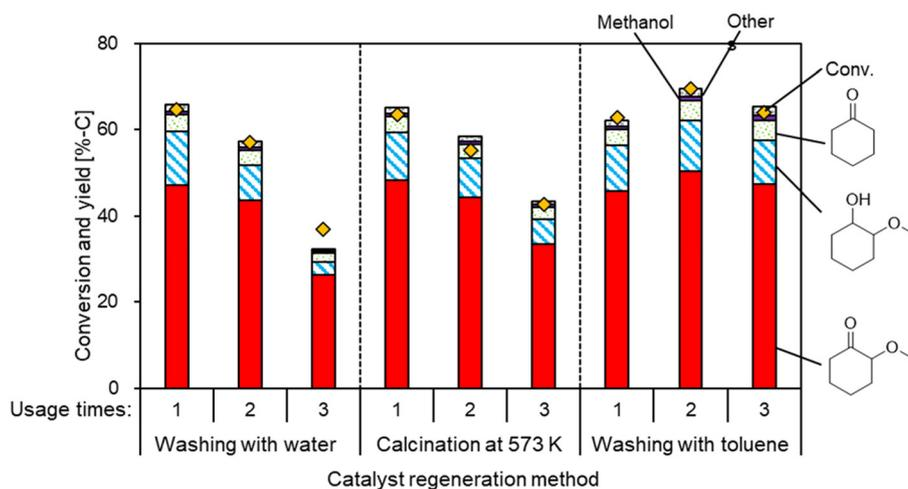
Fig. 8 Reusability of the Pd/TiO<sub>2</sub> catalyst in guaiacol hydrogenation. Conditions: guaiacol (0.62 g), Pd/TiO<sub>2</sub> (Pd = 3 wt%, 200 mg), water (10 g), 373 K, H<sub>2</sub> (1 MPa at r.t.), 4 h.
