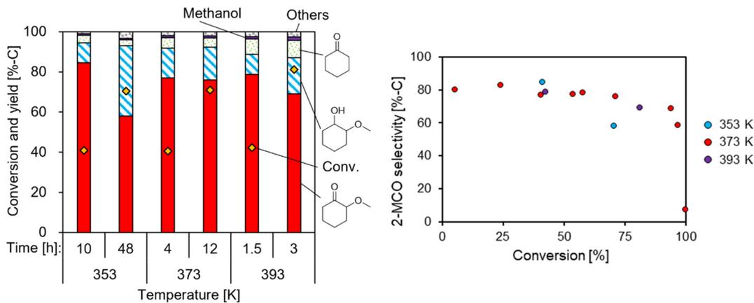
Fig. 7 Effect of reaction temperature and time on the selective hydrogenation of guaiacol over the Pd/TiO<sub>2</sub> catalyst. Conditions: guaiacol (0.62 g), Pd/TiO<sub>2</sub> (Pd = 3 wt%, 100 mg), water (10 g), H<sub>2</sub> (1 MPa at r.t.).
