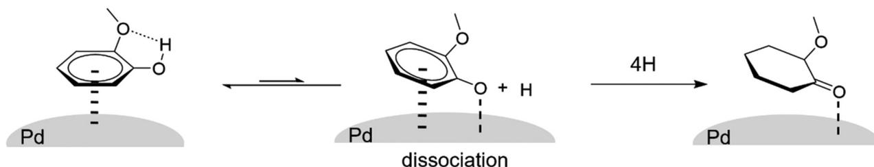
Fig. 9 Possible reaction routes for the selective hydrogenation of guaiacol over the Pd/TiO<sub>2</sub> catalyst in water solvent.
