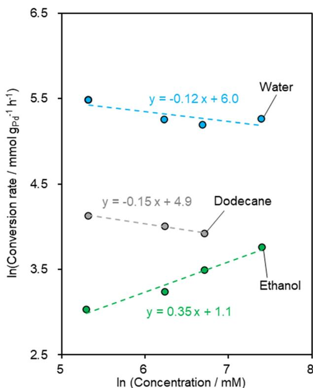
**Fig. 6** Double logarithmic plot of the conversion rate as a function of guaiacol concentration for guaiacol hydrogenation over Pd/TiO<sub>2</sub> in various solvents. Conditions: guaiacol (2–16 mmol), Pd/TiO<sub>2</sub> (Pd = 3 wt%, 100 mg), solvent (10 g), H<sub>2</sub> (1 MPa at r.t.), 373 K.
